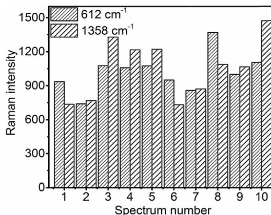
Fig. 9 Raman intensity bar diagram of  $612\text{ cm}^{-1}$  and  $1358\text{ cm}^{-1}$  peaks of R6G in the spike region of various  $\text{MoO}_3$  sea urchins across the substrate at 10 random positions.
