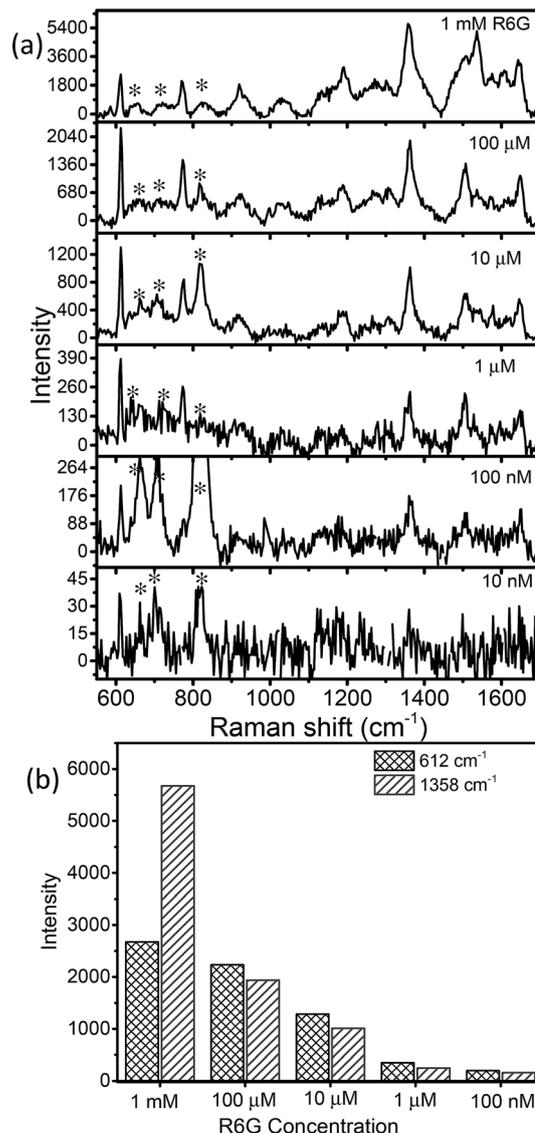
Fig. 7 (a) SERS spectra of various concentrations of R6G coated on MoO<sub>3</sub> sea urchin structures (\* denotes  $\alpha$ -MoO<sub>3</sub> signatures) and (b) plot of R6G concentration versus Raman peak intensity (612 cm<sup>-1</sup> and 1358 cm<sup>-1</sup>).
