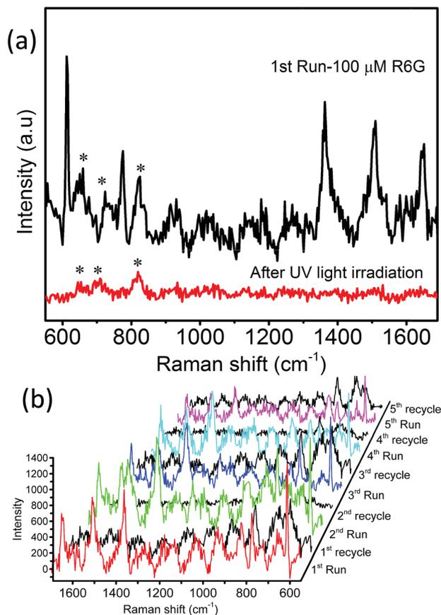
Fig. 10  $\text{MoO}_3$  sea urchins as renewable SERS substrates: (a) SERS of  $100 \mu\text{M}$  R6G before and after UV treatment and (b) reusability of  $\text{MoO}_3$  sea urchin substrates for  $100 \mu\text{M}$  R6G tested for five runs before and after UV treatment (\* denotes  $\alpha\text{-MoO}_3$  peaks).
