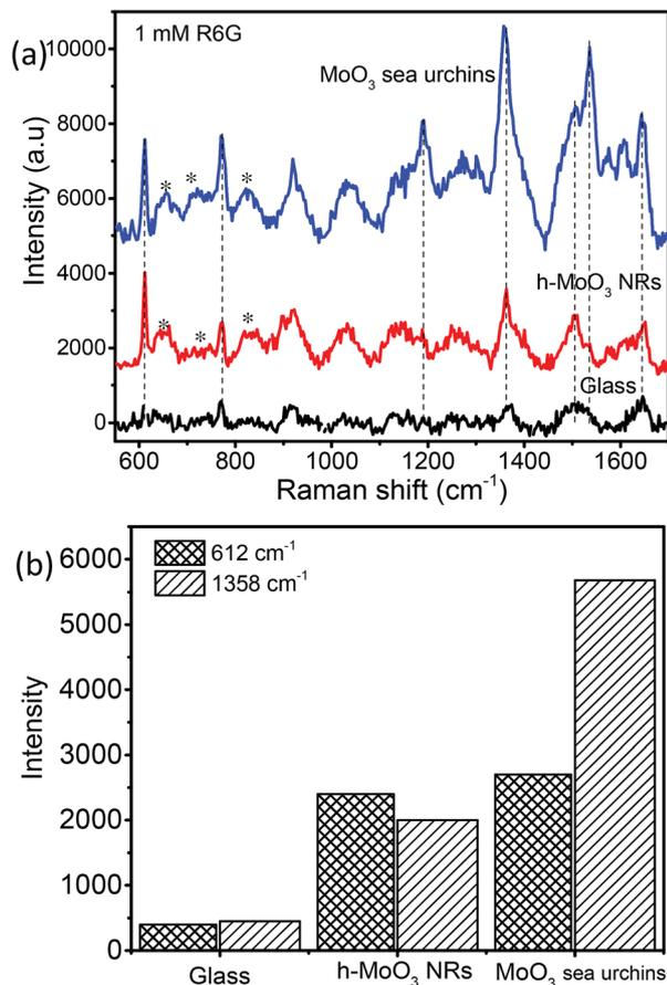
Fig. 6 (a) SERS spectra of 1 mM R6G coated on various substrates on bare glass, h-MoO<sub>3</sub> nanorods/Si and MoO<sub>3</sub> sea urchins/glass and (b) Raman band intensity bar diagram (\* denotes  $\alpha$ -MoO<sub>3</sub> Raman peaks).
