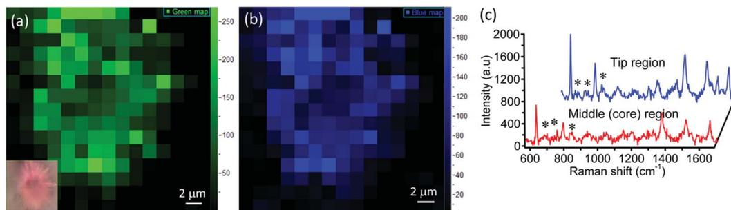
Fig. 8 SERS intensity mapping of 100  $\mu\text{M}$  R6G adsorbed on a single sea urchin  $\text{MoO}_3$  (a)  $612\text{ cm}^{-1}$  peak (green); inset shows the optical image of a single  $\text{MoO}_3$  sea urchin with R6G (b)  $1358\text{ cm}^{-1}$  peak (blue) and (c) SERS spectra of R6G in the tip and middle regions of the  $\text{MoO}_3$  sea urchin nanostructures.
