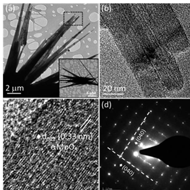
Fig. 4 TEM images of  $\text{MoO}_3$  sea urchins: (a) low magnification image; inset shows the complete view of one sea urchin. (b) High magnification image of (a), (c) HRTEM image of a spine and (d) SAED pattern from the spines of sea urchins.
