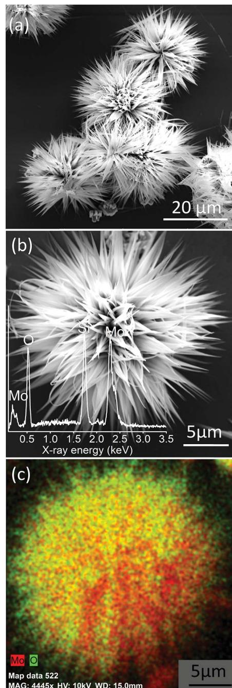
Fig. 1 (a) FESEM images of MoO<sub>3</sub> sea urchins on a Si substrate synthesized by chemical bath deposition, (b) magnified image of a single MoO<sub>3</sub> sea urchin; inset shows the EDS spectra and (c) EDS composite map of Mo L (red) and O K (green) levels from a single sea urchin. Yellow colour is seen due to the overlap of green and red in the same region (see Fig. S3†).
