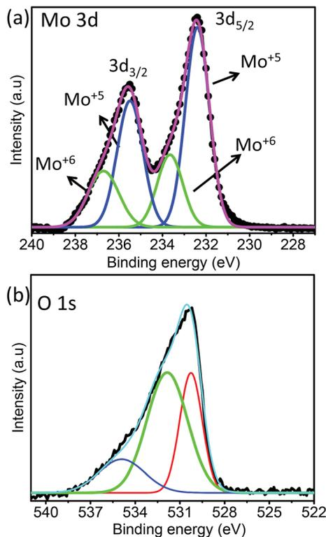
Fig. 5 XPS of MoO<sub>3</sub> sea urchin structures: (a) Mo 3d and (b) O 1s spectra.
