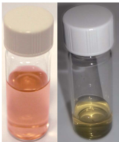
Fig. 2 Sample photographs, left, sample produced by jet co-deposition. This is the colour that essentially all samples had immediately post production. Right, sample produced by jet co-deposition of a silica-methanol solution, after aging approximately three months.
