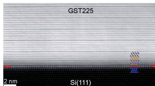
Fig. 8 Atomic-resolution HAADF-HRSTEM image of the interface between the Si(111) substrate and trigonal GST225 thin film. The Sb/Te passivation layer on top of the substrate is marked by red arrows. The insert shows a scheme of the Si-Sb/T-GST225 interface. The Si atoms are marked by blue spheres and the Sb/Te passivation layer is shown by red spheres whereas Te atoms are marked by olive spheres and azure/orange spheres represent Sb/Ge atoms. Due to the slight in-plane rotation of the GST225 crystal structure, the Te, Sb and Ge atomic columns are not resolved in the HAADF image.
