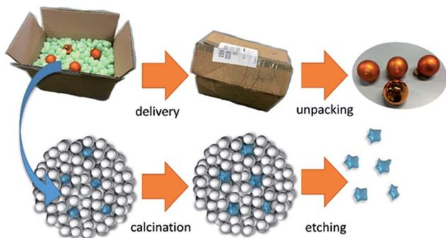
Fig. 1 Similar to foam peanuts, which are used as protectant against mechanical damage in the packaging of fragile products, SiO<sub>2</sub> NPs protect sinter-labile NPs within a supraparticle during calcination.
