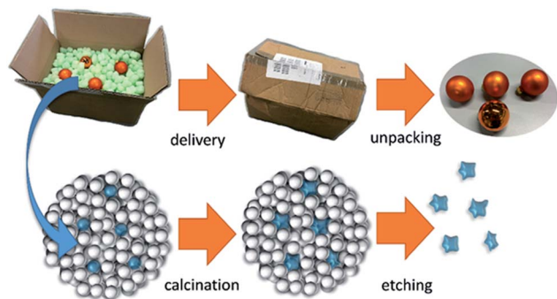
Fig. 1 Similar to foam peanuts, which are used as protectant against mechanical damage in the packaging of fragile products, SiO 2 NPs protect sinter-labile NPs within a supraparticle during calcination.
