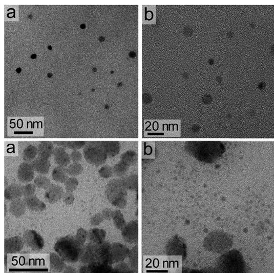
Fig. 4 Transmission electron microscopy (TEM) analyses of the nanocrystals (NCs) after a relatively fast ion exchange reaction: (a and b) cesium bismuth bromide ( $\text{Cs}_3\text{Bi}_2\text{Br}_9$ ) nanocrystals; and (c and d) cesium bismuth chloride ( $\text{Cs}_3\text{Bi}_2\text{Cl}_9$ ) nanocrystals. The average dimensions of the  $\text{Cs}_3\text{Bi}_2\text{Br}_9$  and  $\text{Cs}_3\text{Bi}_2\text{Cl}_9$  NCs increased to  $\sim 12$  nm and  $\sim 22$  nm, respectively.
