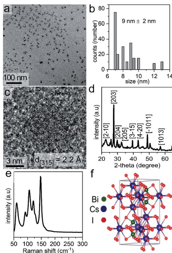
Fig. 1 Cesium bismuth iodide ( $\text{Cs}_3\text{Bi}_2\text{I}_9$ ) nanocrystals (NCs) as characterized by: (a) transmission electron microscopy (TEM) imaging; (b) a histogram of their size distribution obtained from TEM analyses; (c) a high-resolution (HR) TEM analysis; (d) a powder X-ray diffraction analysis; (e) Raman spectroscopy techniques; and (f) a model of the hexagonal crystal structure for  $\text{Cs}_3\text{Bi}_2\text{I}_9$ .
