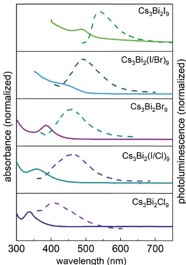
Fig. 5 Absorption (solid) and photoluminescence (dashed) spectra of the perovskite  $\text{Cs}_3\text{Bi}_2\text{I}_9$  NCs, as well as NCs containing  $\text{Br}^-$  and  $\text{Cl}^-$  prepared by the substitution of  $\text{I}^-$  with  $\text{Br}^-$  (2nd and 3rd panels from the top) and  $\text{Cl}^-$  (4th and 5th panels from the top).
