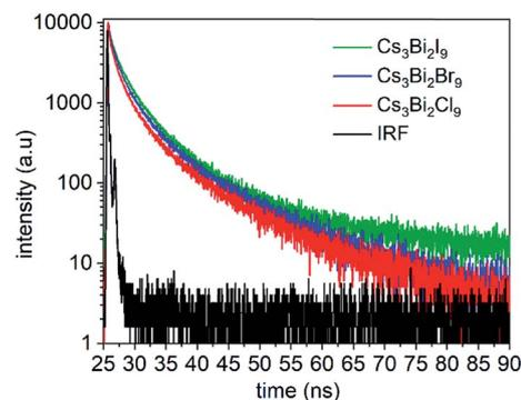
Fig. 6 Time-resolved PL spectra for  $\text{Cs}_3\text{Bi}_2\text{I}_9$  NCs (green),  $\text{Cs}_3\text{Bi}_2\text{Br}_9$  NCs (blue), and  $\text{Cs}_3\text{Bi}_2\text{Cl}_9$  NCs (red) as measured by time-correlated single photon counting (TCSPC) using an excitation wavelength of 370 nm. The instrument response function (IRF) of the TCSPC set-up was measured using a non-fluorescent scatterer, LUDOX®-50.
