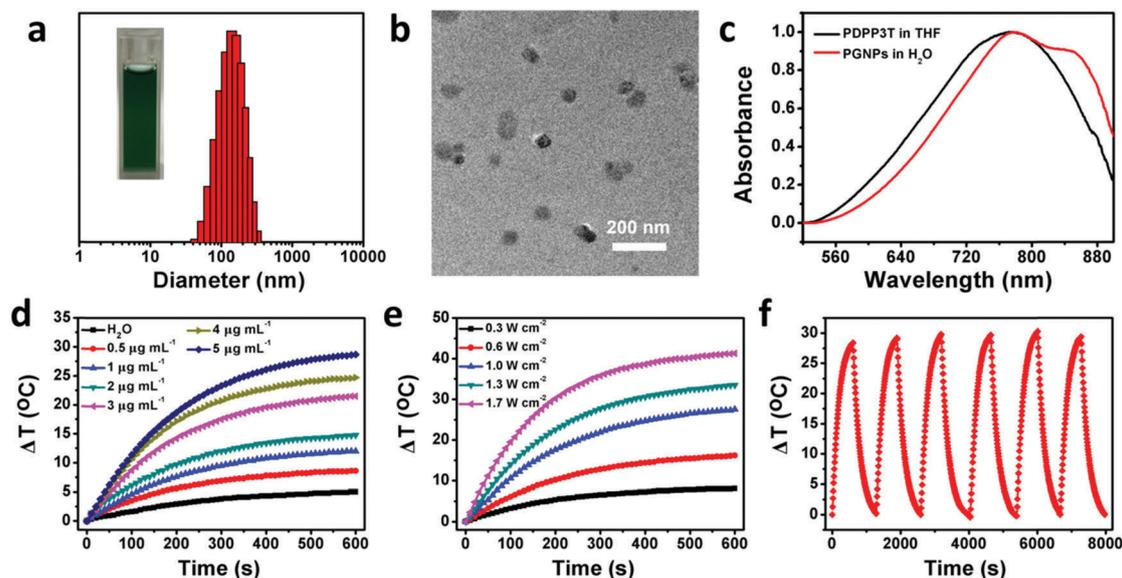
**Fig. 1** Basic characterizations and photothermal performance of PGNPs. (a) DLS result (Inset: Picture of PGNPs in water) and (b) TEM image of PGNPs. (c) Absorption spectra of PDPP3T in THF and PGNPs in water. Photothermal conversion behavior of PGNPs by varying (d) concentrations (0–5 μg mL<sup>-1</sup>) and (e) laser power densities (0.3–1.7 W cm<sup>-2</sup>). (f) Heating reproducibility of PGNPs (5 μg mL<sup>-1</sup>) in water over 6 cycles of heating-cooling.
