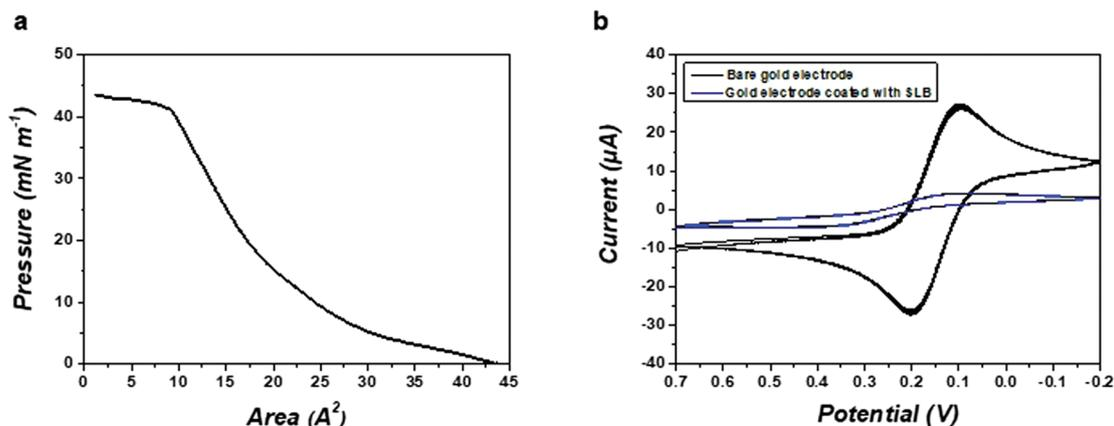
**Fig. 2** Characterization of the SLB assembled on the integrated microchip. (a)  $\pi$ - $A$  compression isotherm of POPG at the air–water interface at room temperature. (b) CV responses of  $1 \text{ mM K}_3\text{Fe}(\text{CN})_6$  in  $1 \text{ M KCl}$  at the embedded gold electrode of the integrated microchip (black: bare electrode without SLB, blue: electrode coated with the SLB).
