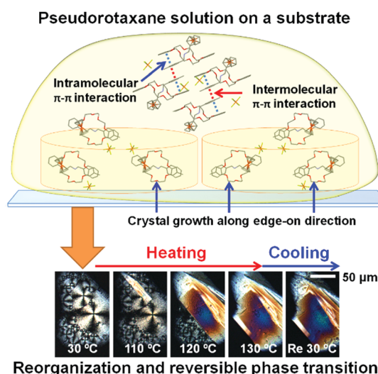
Fig. 11 Schematic illustration of the film formation and optical micrographs of a film of 1 under polarized light. The figure was modified using ref. 85 and reprinted with permission from the Royal Society of Chemistry, Copyright (2014).
