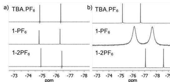
**Fig. 3** <sup>19</sup>F NMR of the PF<sub>6</sub><sup>-</sup> salts in (a) acetonitrile-*d*<sub>3</sub> and (b) chloroform-*d*.
