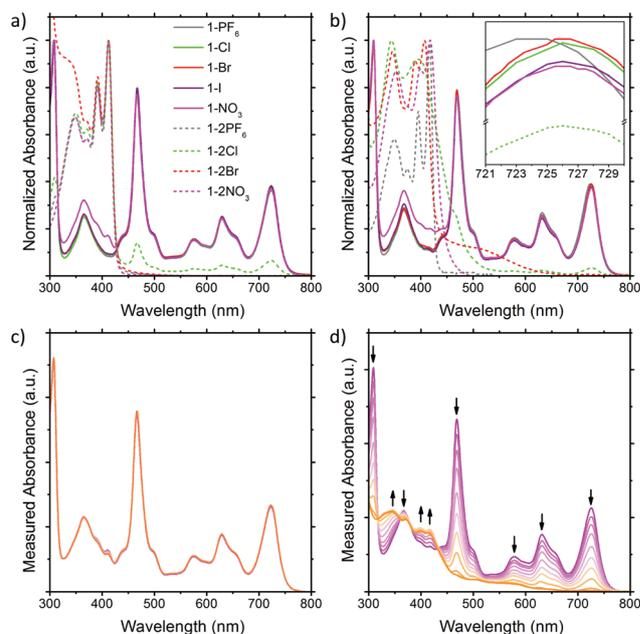
**Fig. 2** Solution UV-Vis of the BTTPP-NDI salts in (a) acetonitrile and (b) chloroform. Solution UV-Vis of **1-NO<sub>3</sub>** in (c) acetonitrile and (d) chloroform upon illumination.
