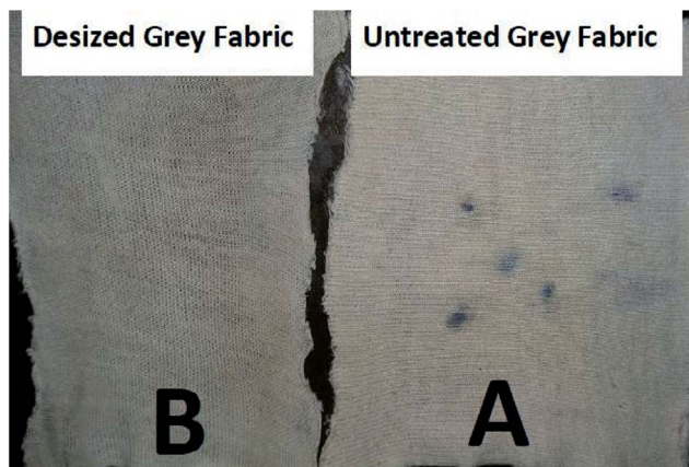
Fig. 10 Assessment of the desizing potential of recombinant \alpha -amylase enzyme on grey fabric: (A) the spots present on untreated grey fabric are purple, (B) no spot on the desized fabric.
