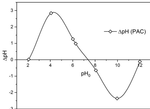
Fig. 1 Determination of  $\text{pH}_{\text{pzc}}$  for PAC.
