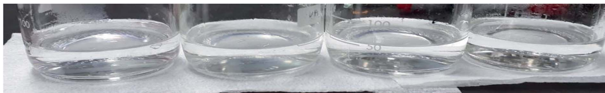
Fig. 5 Clarity of the 50 : 30 : 20 ECH/IPA/water (w/w) feed mixture solution after 15 days of immersion.
