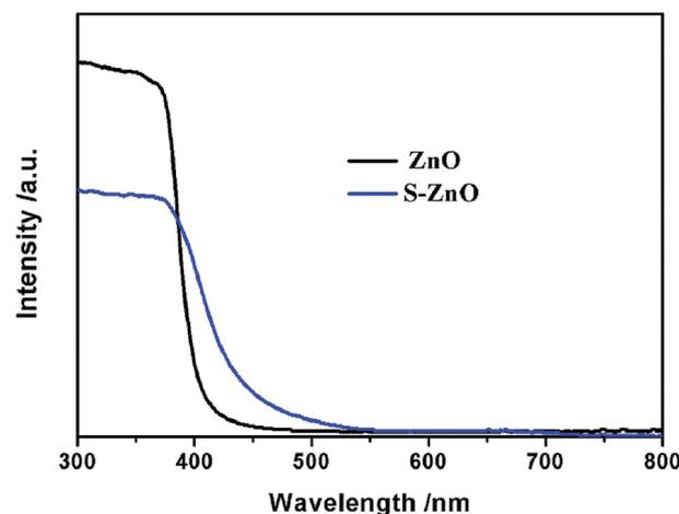
Fig. 4 The UV-Vis-NIR spectra of ZnO and S-ZnO.
