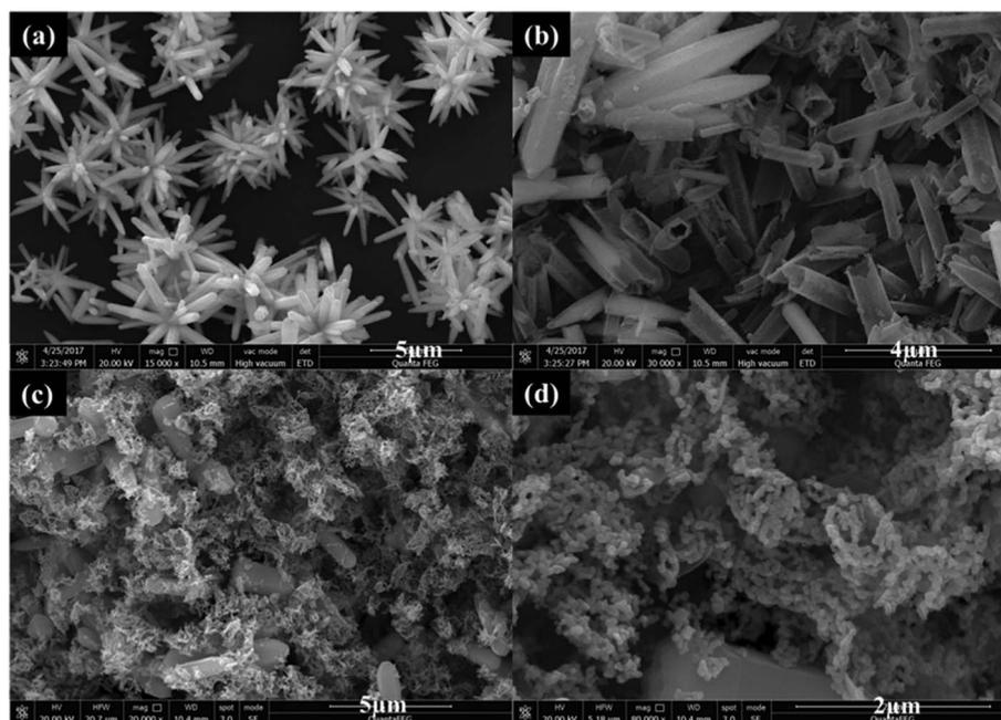
Fig. 2 FESEM images of (a) ZnO after treating with  $\text{Na}_2\text{S}$ , (b) ZnO after treating with NaOH, (c and d) S-ZnO.
