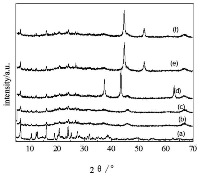
Fig. 2 XRD patterns of (a) fresh FCC catalyst, (b) spent FCC catalyst, (c) calcined spent FCC catalyst, (d) supported NiO catalyst, (e) supported Ni catalyst and (f) used Ni loaded catalyst.
