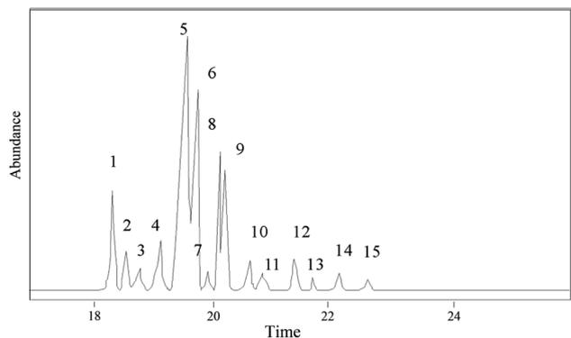
Fig. 10 GC-MS chromatogram of methylated acid fraction in hydrogenated rosin.
