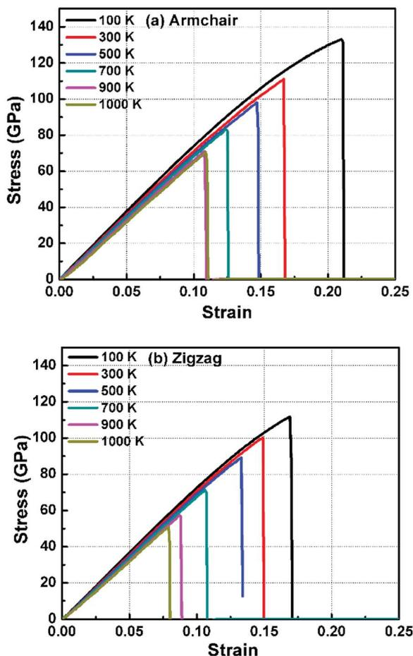
Fig. 5 The Illustration of the temperature dependence of the stress–strain response of h-BCN sheet under uniaxial tension along (a) armchair and (b) zigzag direction at a strain rate of  $0.001 \text{ ps}^{-1}$ .
