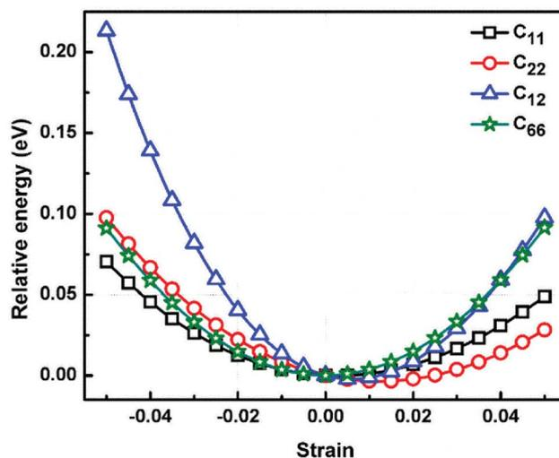
**Fig. 4** The relative energy versus strain response graph of h-BCN sheet using molecular statics simulations for the analysis of elastic constants. The relative energy is plotted as a function of various specific strains necessary for calculating the elastic tensors.
