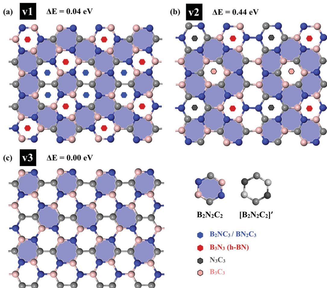
Fig. 1 Three possible h-BCN monolayers structures, namely (a) h-BCN\_v1, (b) h-BCN\_v2 and (c) h-BCN\_v3 with relative stability.
