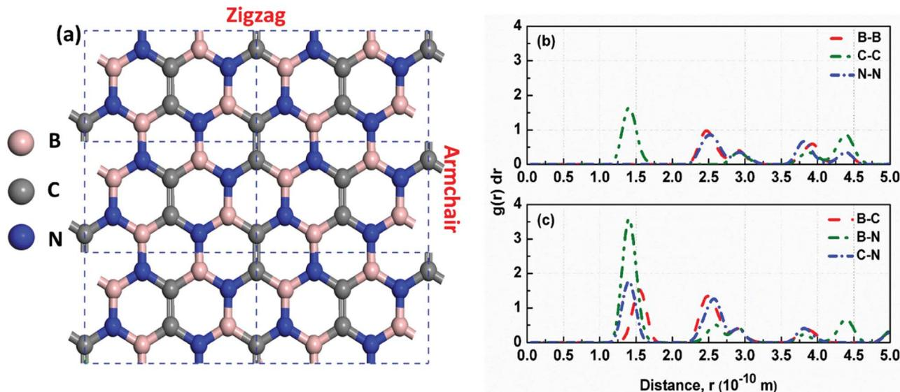
Fig. 2 (a) The optimized structure of h-BCN<sub>v3</sub> monolayer. The dashed black rectangles represent the unit cell of h-BCN with a lattice constant of 7.59 Å; (b) and (c) Radial distribution function of B–B, C–C, N–N, B–C, B–N and C–N pairs in a h-BCN sheet at 300 K. The value of RDF at any  $r$  decreases as the temperature increases due to thermal broadening.
