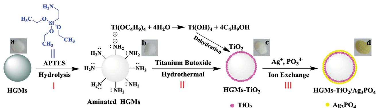
Fig. 1 Schematic illustration of the fabrication process of floating HGMS- $\text{TiO}_2/\text{Ag}_3\text{PO}_4$  composite. (Inset: digital photos of HGMS (a), aminated HGMS (b), HGMS- $\text{TiO}_2$  (c) and HGMS- $\text{TiO}_2/\text{Ag}_3\text{PO}_4$  (d)).
