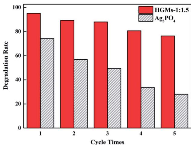
Fig. 7 Cycling runs of the  $5 \text{ mg L}^{-1}$  MB photo-degradation at the presence of  $2 \text{ g L}^{-1}$  HGMS-1 : 1.5.
