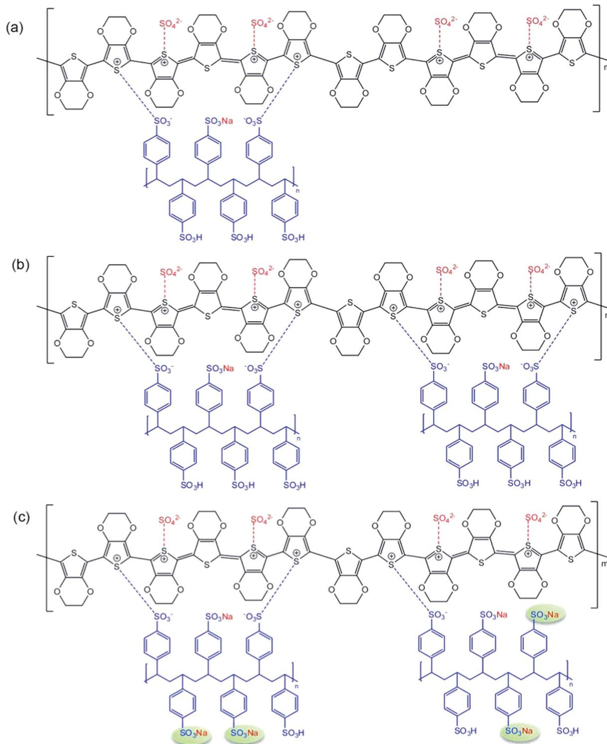
**Scheme 2** Proposed interaction of PEDOT:PSS at the EDOT :  $\text{Na}_2\text{S}_2\text{O}_8$  mole ratio of 1 : 1 and various EDOT : PSS weight ratios: at an EDOT : PSS weight ratio (a) lower than 1 : 11, (b) 1 : 11, where more PSS interact, and (c) higher than 1 : 11 with a higher PSSNa amount to reduce the doping sites on PSS.
