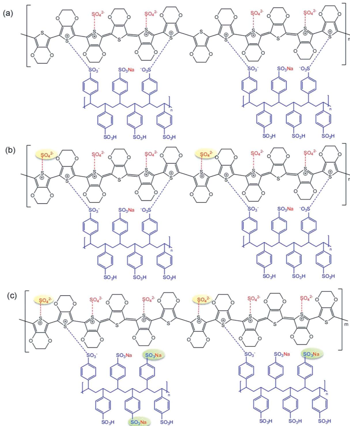
**Scheme 3** Proposed structure of PEDOT:PSS at the EDOT : PSS weight ratio of 1 : 11 and at various EDOT : Na<sub>2</sub>S<sub>2</sub>O<sub>8</sub> mole ratios: at an EDOT : Na<sub>2</sub>S<sub>2</sub>O<sub>8</sub> mole ratio (a) lower than 1 : 2, (b) 1 : 2, where SO<sub>4</sub><sup>2-</sup> acts as a secondary dopant and (c) higher than 1 : 2, where a higher PSSNa amount is generated.
