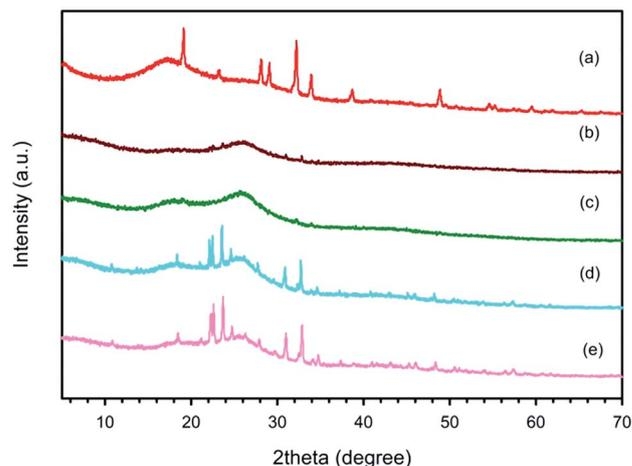
Fig. 3 XRD spectra of commercial PSSNa and PEDOT:PSS at the EDOT : PSS weight ratio of 1 : 11 and at various EDOT : Na<sub>2</sub>S<sub>2</sub>O<sub>8</sub> mole ratios: (a) PSSNa, and EDOT : Na<sub>2</sub>S<sub>2</sub>O<sub>8</sub> mole ratio of (b) 1 : 1, (c) 1 : 2, (d) 1 : 3 and (e) 1 : 4.
