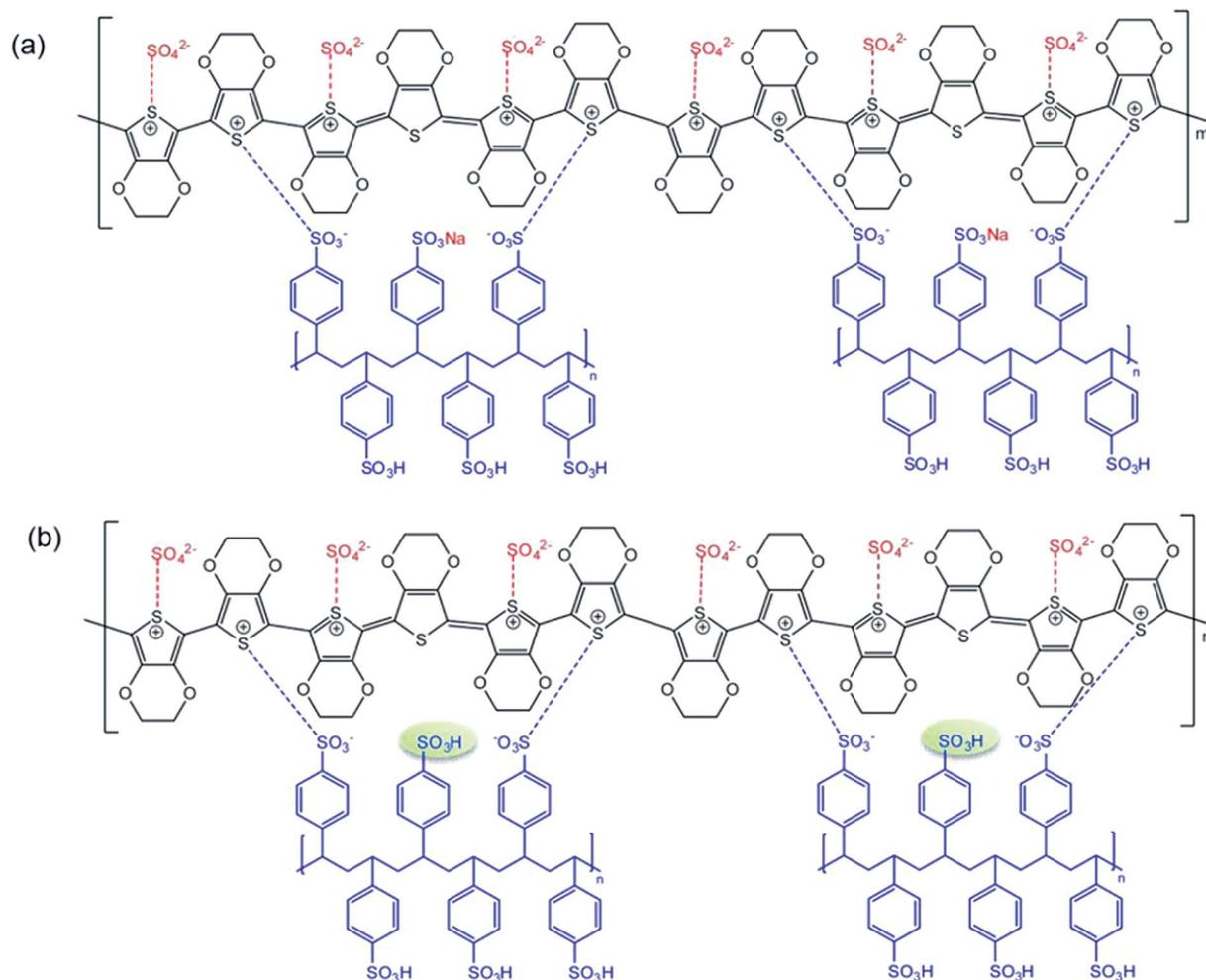
**Scheme 4** Proposed structure of PEDOT:PSS at the EDOT : PSS weight ratio of 1 : 11 and EDOT :  $\text{Na}_2\text{S}_2\text{O}_8$  mole ratio of 1 : 2: (a) no surfactant; and (b) Triton X-100, where PSSNa amount is reduced through methanol washing.
