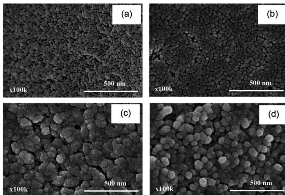
Fig. 6 PEDOT:PSS surface morphology at the EDOT : PSS weight ratio of 1 : 11 and EDOT : Na<sub>2</sub>S<sub>2</sub>O<sub>8</sub> mole ratio of 1 : 2 using various surfactant types: (a) no surfactant, (b) CTAB (2.5CMC), (c) SDS (2.5CMC), and (d) Triton X-100 (2.5CMC).
