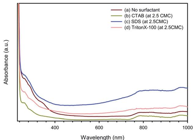
Fig. 4 UV adsorption spectra of PEDOT:PSS at the EDOT : PSS weight ratio of 1 : 11 and EDOT : Na<sub>2</sub>S<sub>2</sub>O<sub>8</sub> mole ratio of 1 : 2 using various surfactant types: (a) no surfactant, (b) CTAB (at 2.5CMC), (c) SDS (at 2.5CMC), and (d) Triton X-100 (at 2.5CMC).
