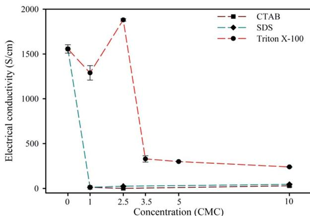
Fig. 10 Electrical conductivity of PEDOT:PSS at the EDOT : PSS weight ratio of 1 : 11 and EDOT : Na<sub>2</sub>S<sub>2</sub>O<sub>8</sub> mole ratio of 1 : 2 with various surfactant types and concentrations.
