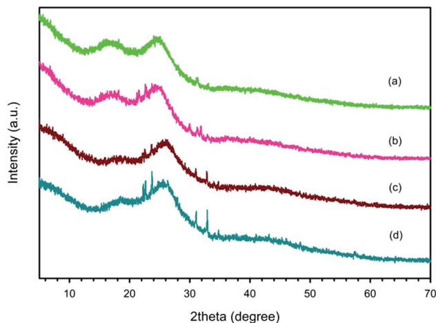
Fig. 2 XRD spectra of PEDOT:PSS at the EDOT : Na<sub>2</sub>S<sub>2</sub>O<sub>8</sub> mole ratio of 1 : 1 and at various EDOT : PSS weight ratios: (a) EDOT : PSS weight ratio of 1 : 1, (b) EDOT : PSS weight ratio of 1 : 5, (c) EDOT : PSS weight ratio of 1 : 11, and (d) EDOT : PSS weight ratio of 1 : 13.
