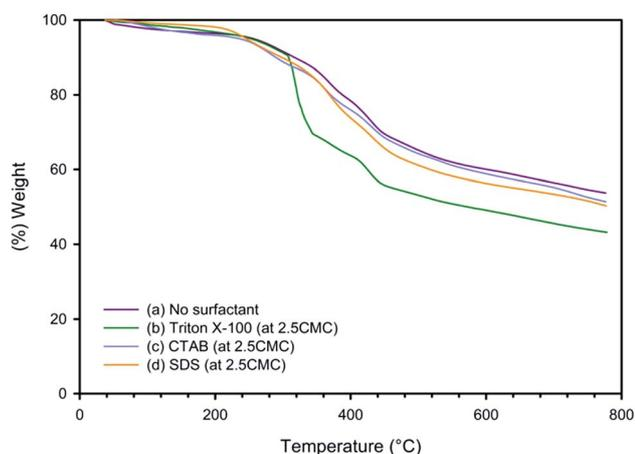
Fig. 7 TGA spectra of PEDOT:PSS at the EDOT : PSS weight ratio of 1 : 11 and EDOT :  $\text{Na}_2\text{S}_2\text{O}_8$  mole ratio of 1 : 2: (a) no surfactant, (b) Triton X-100 (2.5CMC), (c) CTAB (2.5CMC) and (d) SDS (2.5CMC).
