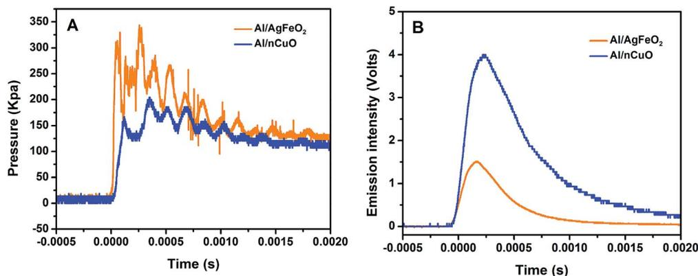
Fig. 6 Temporal pressure and optical behavior of Al/AgFeO<sub>2</sub> and Al/nCuO.Table 3 Thermodynamic equilibrium predictions of Al/CuO, Al/Ag<sub>2</sub>O and Al/Fe<sub>2</sub>O<sub>3</sub> thermites<sup>a</sup>
