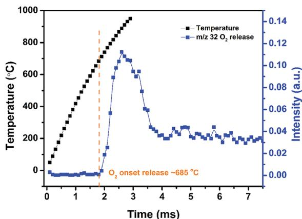
Fig. 3 Temperature and  $\text{O}_2$  temporal profile of  $\text{AgFeO}_2$ .
