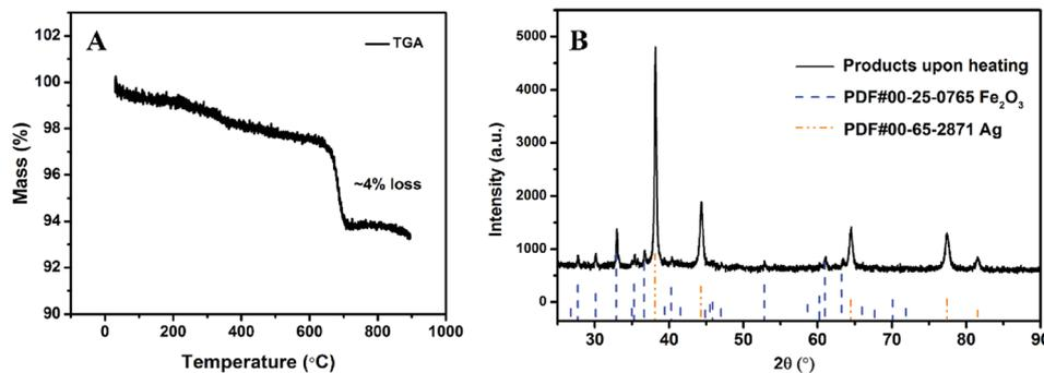
Fig. 2 (A) TGA of  $\text{AgFeO}_2$  in Ar at a heating rate of  $10\text{ °C min}^{-1}$ ; (B)  $\text{AgFeO}_2$  decomposition product after heating to  $1000\text{ °C}$ .
