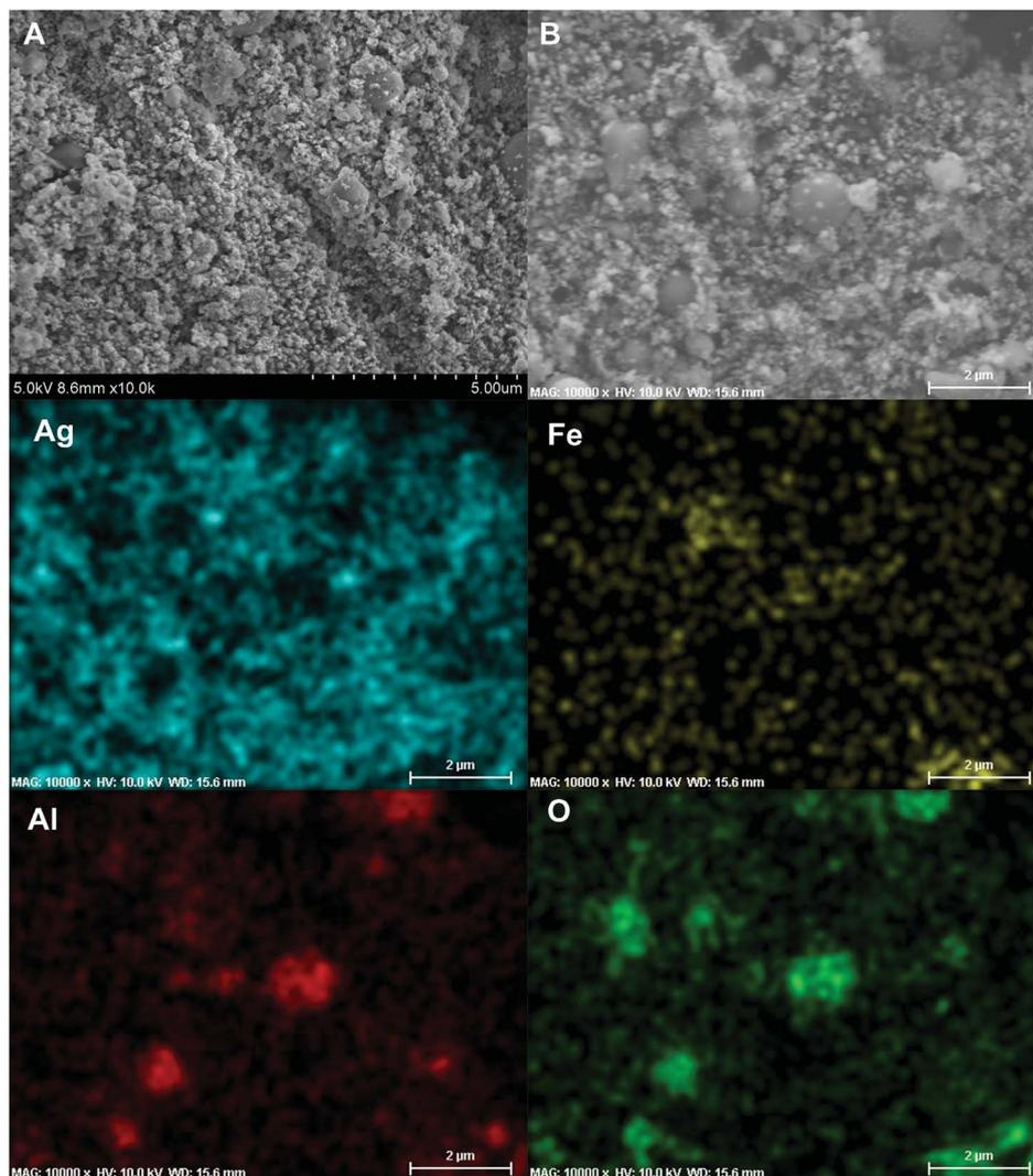
Fig. 8 Representative SEM images (A and B) of the Al/AgFeO<sub>2</sub> reaction product collected inside the combustion cell; 2D elemental mapping (Ag, Fe, Al and O) of (B) using EDS.
