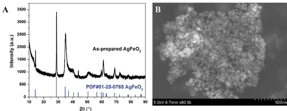
Fig. 1 XRD spectrum (A) and SEM image (B) of AgFeO<sub>2</sub> prepared via co-precipitation.
