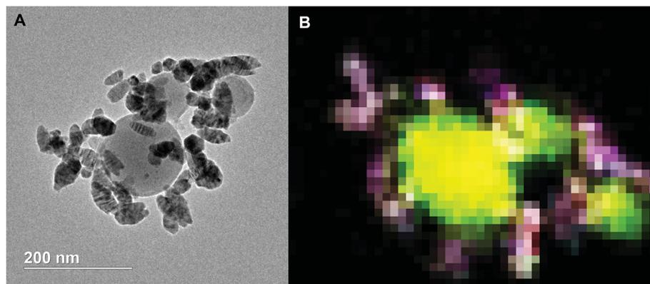
Fig. 9 TEM image (A) and 2D elemental mapping (B) of the Al/AgFeO<sub>2</sub> reaction product. Red represents Ag, blue represents Fe, yellow represents Al and green represents O.
