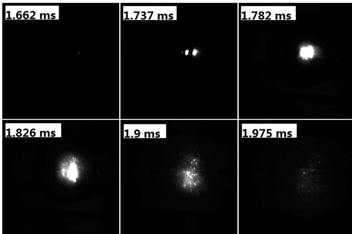
Fig. 4 Sequential snapshots of Al/AgFeO<sub>2</sub> burning on a high-rate heating Pt wire in T-Jump chamber (in vacuum). The labels in each image are the time elapse after triggering.
