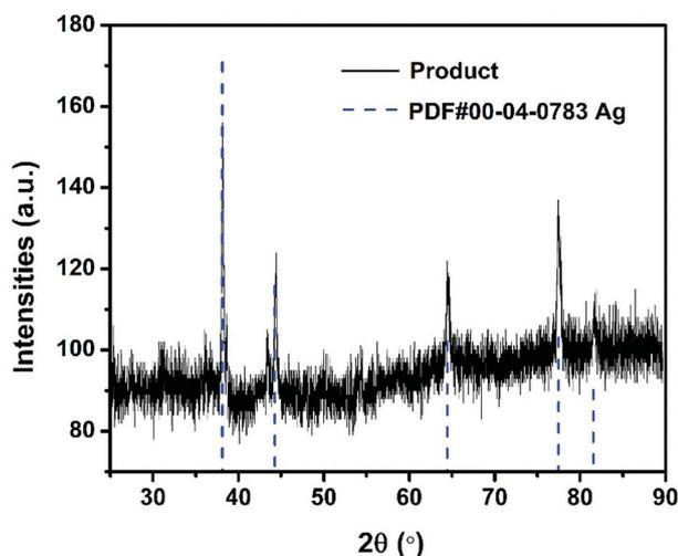
Fig. 7 The XRD pattern of Al/AgFeO<sub>2</sub> reaction product.
