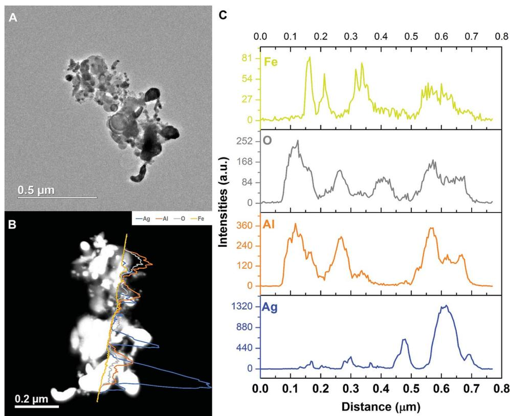
Fig. 10 Representative TEM image and the corresponding EDS line-scan data of the Al/AgFeO<sub>2</sub> reaction product.
