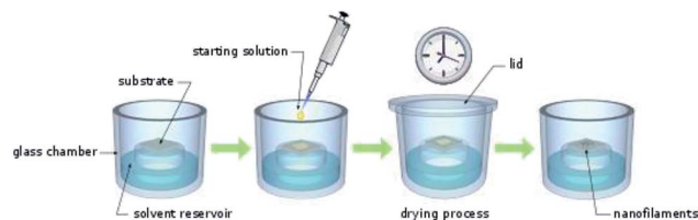
Fig. 1 Schematic of the drying under solvent atmosphere (DUSA) technique. A glass chamber with reservoir and a central, protruded plateau was filled with solvent. A substrate was placed on top of the plateau. Once the atmosphere had saturated, the starting solution (0.01–1 \mu\text{M} in trichloromethane) was deposited onto the substrate. After waiting minutes to days, the droplet had dried and various self-assembled aggregation products (nanowires with different morphology) were found on the substrate surface.
