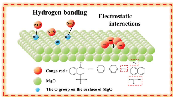
Fig. 5 Schematic diagram of CR on MgO nanoparticles through hydrogen bonding and electrostatic interactions.
