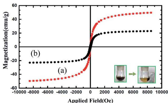
Fig. 3 Magnetization loop of (a)  $\text{Fe}_3\text{O}_4$  and (b)  $\text{Fe}_3\text{O}_4$ @nano-cellulose/Cu(II).
