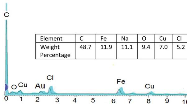
Fig. 5 EDS (EDX) spectra of Fe<sub>3</sub>O<sub>4</sub>@nano-cellulose/Cu(II).
