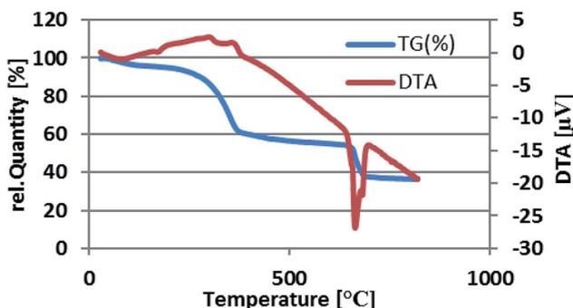
Fig. 6 Thermal gravimetric analysis pattern of Fe<sub>3</sub>O<sub>4</sub>@nano-cellulose/Cu(II).
