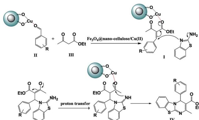
**Scheme 2** Proposed mechanism for the synthesis of 4*H*-pyrimido[2,1-*b*]benzothiazole derivatives IV<sub>a–m</sub>.
