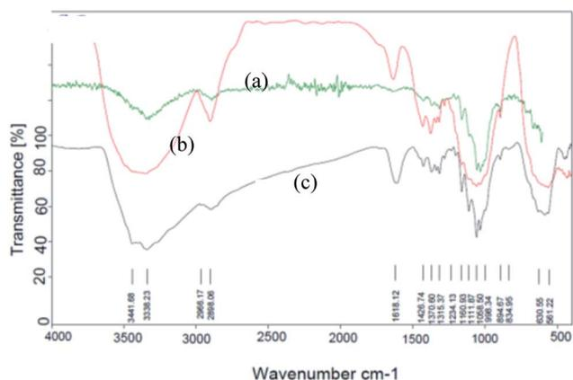
Fig. 1 FT-IR spectra of (a) nano-cellulose, (b)  $\text{Fe}_3\text{O}_4$  @ nano-cellulose and (c)  $\text{Fe}_3\text{O}_4$ @nano-cellulose/Cu(II).
