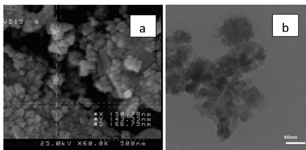
Fig. 4 (a) FESEM image of Fe<sub>3</sub>O<sub>4</sub>@nano-cellulose/Cu(II) and (b) TEM of Fe<sub>3</sub>O<sub>4</sub>@nano-cellulose/Cu(II).
