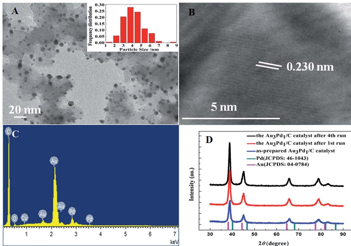
Fig. 1 (A) TEM image with the particle size distribution, (B) HR-TEM image, and (C) EDX spectrum of the newly prepared  $\text{Au}_3\text{Pd}_1/\text{C}$  catalyst. (D) XRD patterns of the newly prepared and recovered  $\text{Au}_3\text{Pd}_1/\text{C}$  catalysts after different experimental runs.
