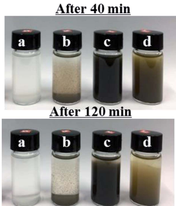
Fig. 4 Photographs of (a) LDHs, (b) Ag-LDHs(PVP), (c) Ag-LDHs@PDA and (d) Ag-LDHs@TA-Fe(III) dispersions after standing for 120 min.
