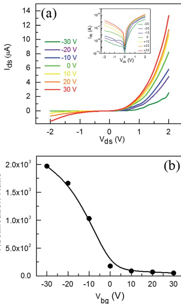
Fig. 2 (a) Gate-dependent rectifying effect of MoTe<sub>2</sub> Schottky junction between Cr/Au-Pd/Au contacts. (b) Rectification ratio as a function of the back gate of MoTe<sub>2</sub> Schottky junction.
