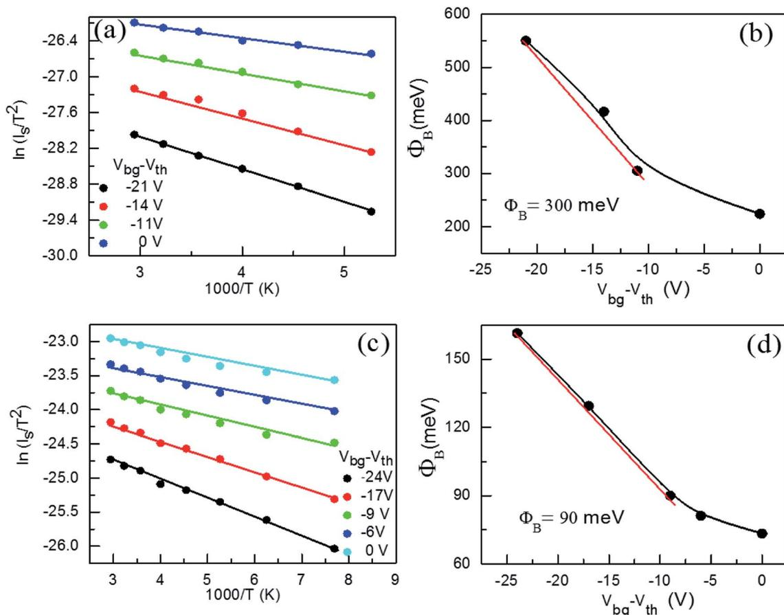
Fig. 3 (a) Conventional Richardson plot  $\ln(I_S/T^2)$  *versus*  $1000/T$  for Cr/Au metal contacts. (b) The potential barrier height at the MoTe<sub>2</sub>/Cr/Au junction as a function of  $V_{\text{bg}} - V_{\text{th}}$ . (c) Conventional Richardson plot  $\ln(I_S/T^2)$  *versus*  $1000/T$  for Pd/Au metal contacts. (d) The potential barrier height at the MoTe<sub>2</sub>/Pd/Au junction as a function of  $V_{\text{bg}} - V_{\text{th}}$ .
