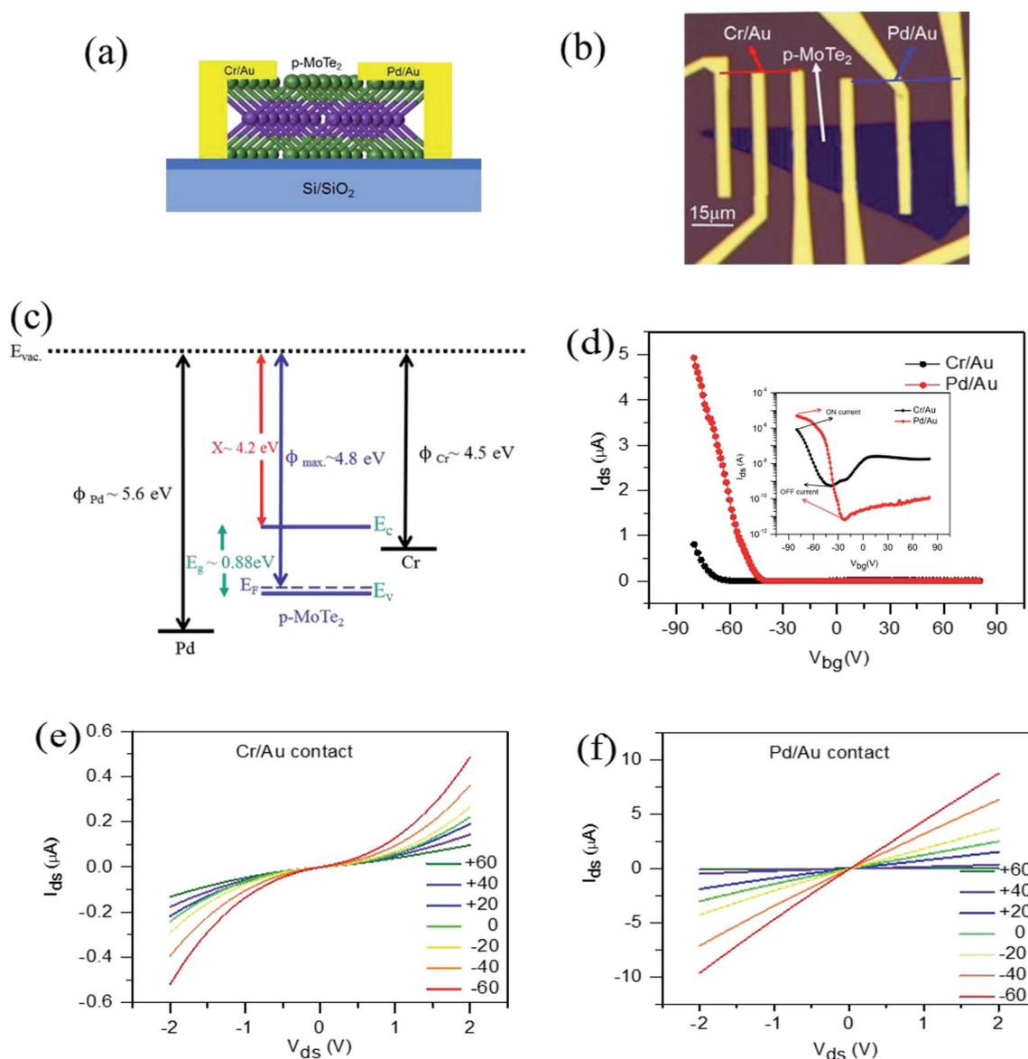
**Fig. 1** (a) Schematic illustration of the MoTe<sub>2</sub> Schottky diode. (b) Optical microscope image of the device. (c) Band profile of Pd/MoTe<sub>2</sub>/Cr. (d) Transfer characteristics of p-MoTe<sub>2</sub> with Pd/Au and Cr/Au FETs with  $V_{ds} = 0.5$  V. The  $I_D$ - $V_D$  characteristics as a function of gate bias, (e) ultra-high resistive metal contact effect of p-MoTe<sub>2</sub> with Cr/Au, and (f) ultra-low resistive ohmic metal contact behavior of MoTe<sub>2</sub> with Pd/Au.
