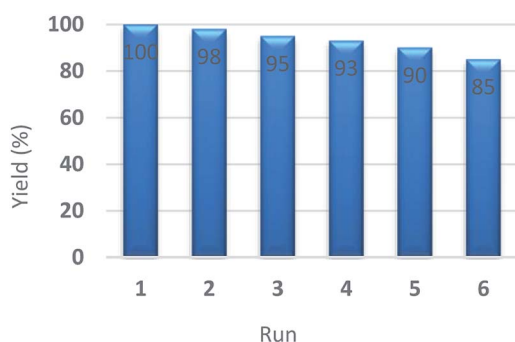
Fig. 6 The recycling efficiency of Pd–NHC–γ-Fe 2 O 3 – n -butyl-SO 3 H in the reduction of nitrobenzene.
