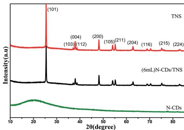
Fig. 1 XRD pattern of N-CDs, TNS and N-CDs/TNS.
