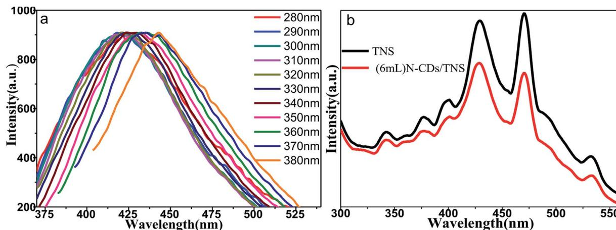
Fig. 6 (a) Normalized fluorescence emission spectra of water solutions of N-CDs acquired using various excitation wavelengths. (b) PL spectra of TNS and (6 mL) N-CDs/TNS.
