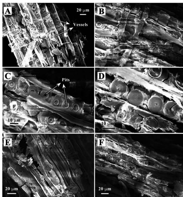
Fig. 2 SEM images of TiO<sub>2</sub>/C material containing biomimetic channels prepared by a wood template after sintering at 400 °C (A–D), 500 °C (E) and 600 °C (F).
