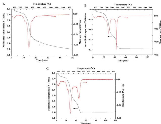
Fig. 6 TGA curves of wood samples impregnated with TiO<sub>2</sub> and catalyst precursors. (A) Constant temperature at 400 °C for 1 hour under air atmosphere; (B) 500 °C; (C) 600 °C.
