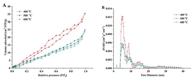
Fig. 4 Nitrogen adsorption/desorption isotherm curves (A) and corresponding pore-size distribution curves (B) of prepared TiO<sub>2</sub> materials under different sintering temperatures.
