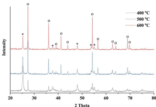
Fig. 3 XRD patterns of the obtained TiO<sub>2</sub> material sintered at 400, 500 and 600 °C for 4 hours (o denotes rutile phase and \* denotes anatase phase).
