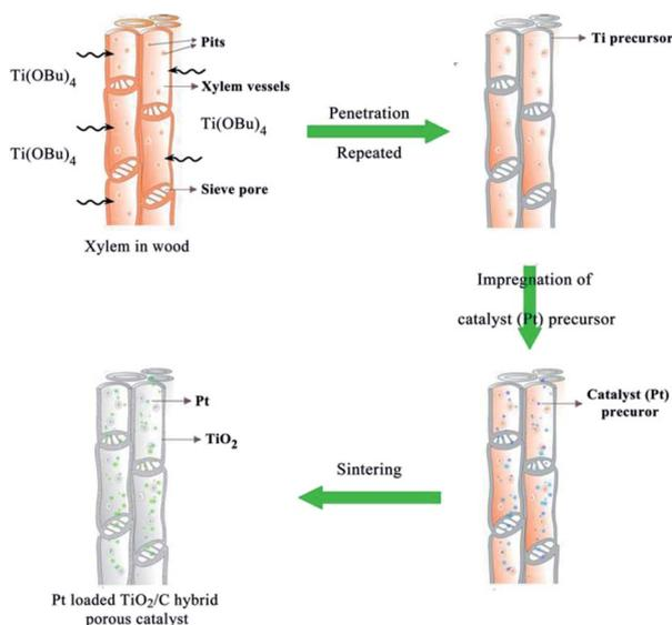
Fig. 1 Schematic illustration of wood templated biomimetic TiO<sub>2</sub>/C hybrid material preparation.
