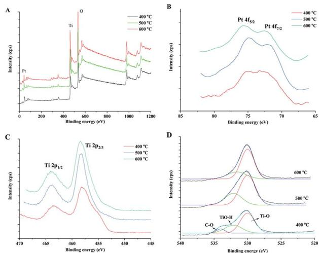
Fig. 5 XPS survey spectra (A) of the obtained catalysts and high resolution spectra of Pt 4f (B), Ti 2p (C) and O 1s (D) of prepared TiO<sub>2</sub> samples under different sintering temperatures.
