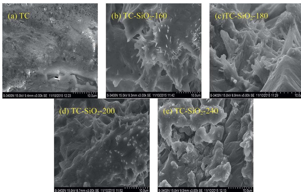
Fig. 3 SEM images of the pure TC (a) and the TC nanofluids: TC-SiO<sub>2</sub>-160 (b), TC-SiO<sub>2</sub>-180 (c), TC-SiO<sub>2</sub>-200 (d), and TC-SiO<sub>2</sub>-240 (e).
