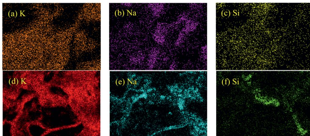
Fig. 2 EDS element mapping images of the TC-SiO<sub>2</sub>-180 (a–c) and TC-SiO<sub>2</sub>-240 (d–f).
