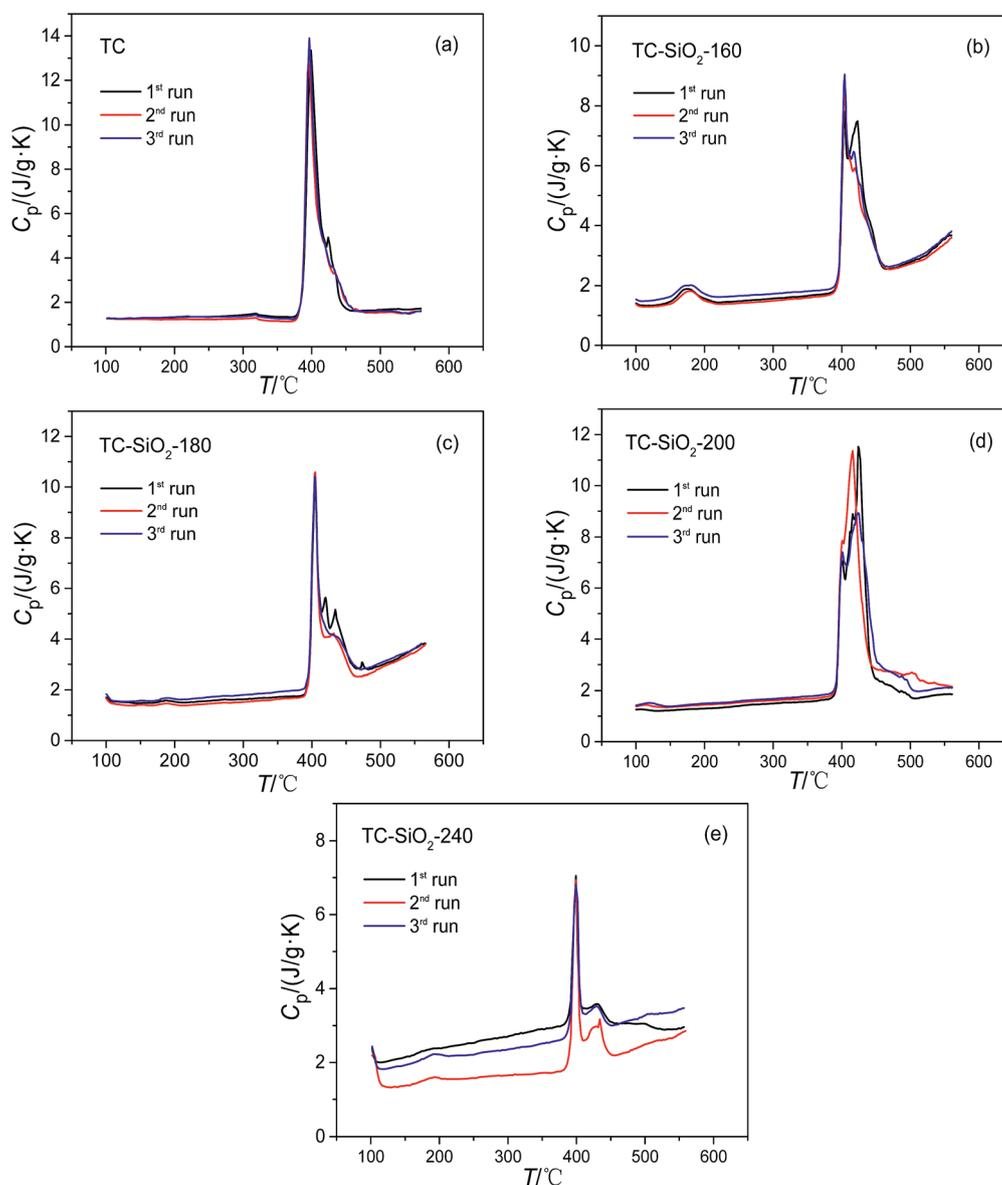
Fig. 1 Variation of specific heat capacity with temperature for the TC (a), and the TC nanofluids with SiO<sub>2</sub> nanoparticles prepared at an evaporation temperature of 160 °C (b), 180 °C (c), 200 °C (d), and 240 °C (e).
