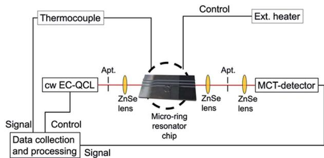
Fig. 3 Scheme of the experimental setup comprising a cw EC-QCL, a MCT-detector, an external heating system, and a thermocouple. Incident radiation is shaped *via* apertures and focused onto the waveguide facet using zinc selenide (ZnSe) lenses. Micro-ring resonator chip, electrical heater, and the thermocouple are in thermal contact.
