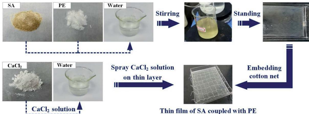
Fig. 1 The preparation process of PECSA film.
