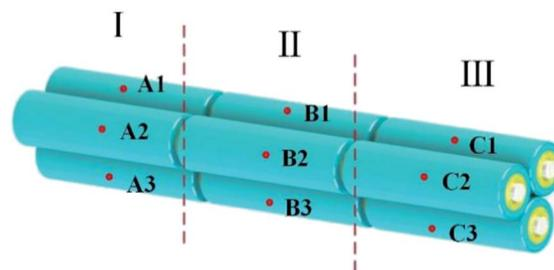
Fig. 3 Distribution of collection points on battery packs.
