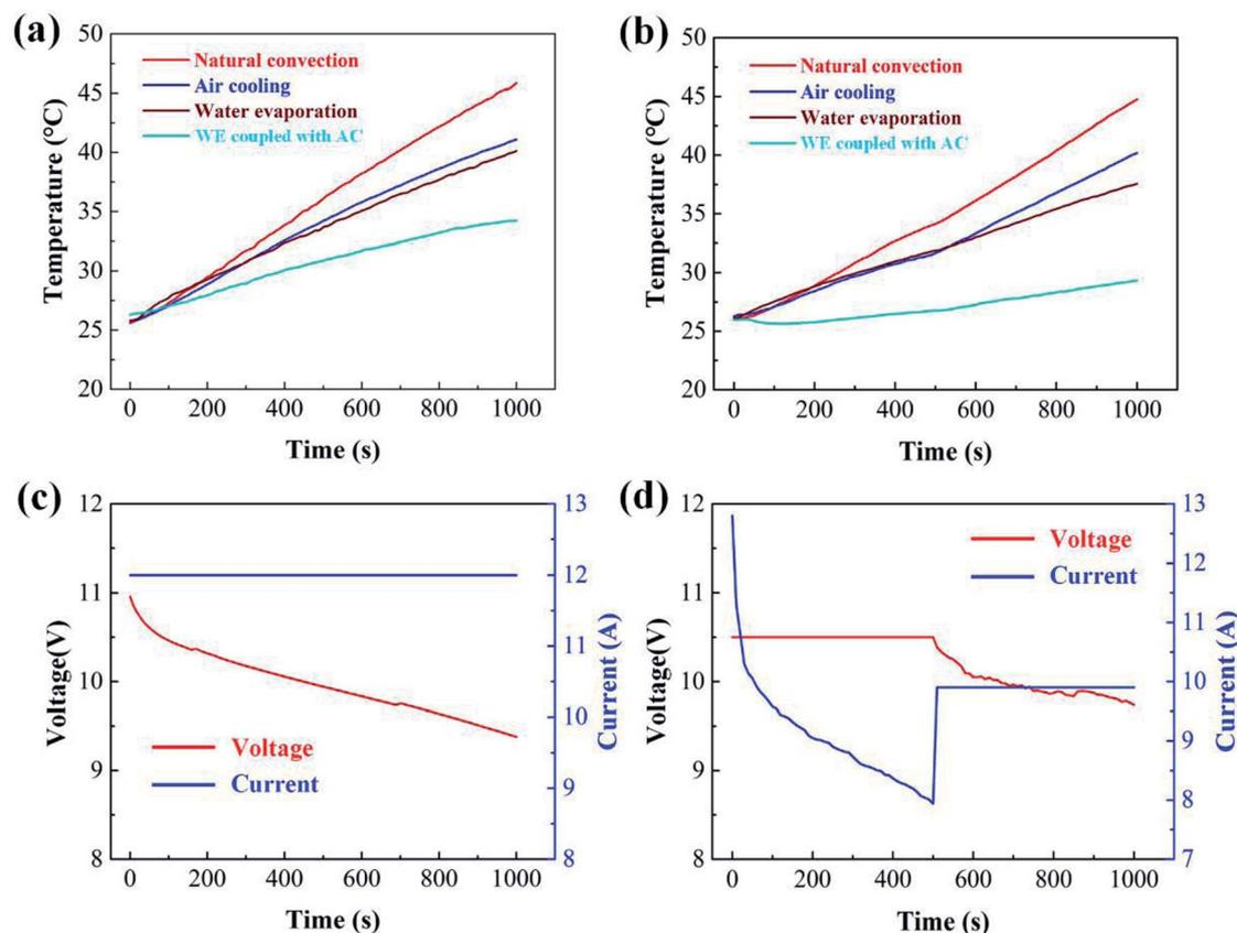
Fig. 9 Temperature of battery on discharge rate of 1.8C and CV + CC.
