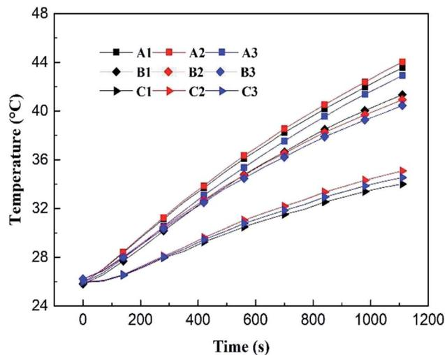
Fig. 4 Battery temperature of different collection points at discharge rate of 1.5C.
