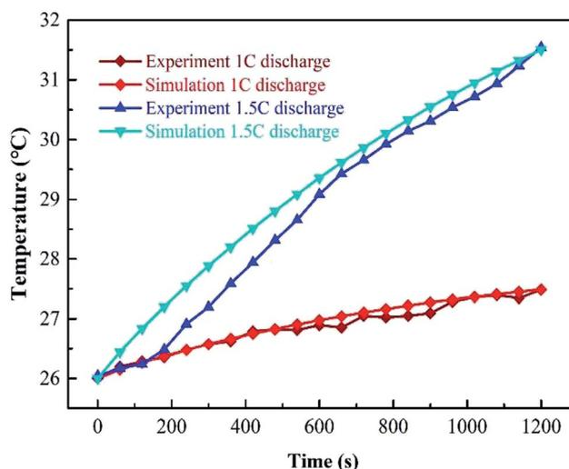
Fig. 6 Comparison between experiment and simulation at 1C and 1.5C when WE is used with AC at an air flow rate of 3 m s<sup>-1</sup>.
