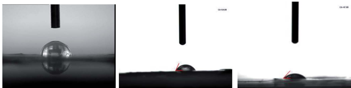
Fig. 6 Surface contact angles of the PSf membrane, AA-PSf membrane and SHPCS-AA-PSf membrane.
