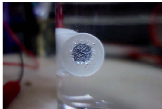
Fig. 5 Oxygen evolution on the sample surface during the galvanostatic polarization test in blank solution.
