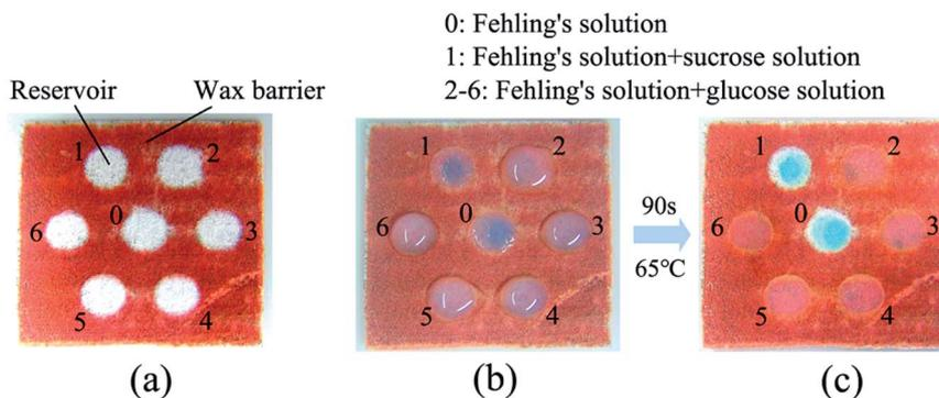
Fig. 6 The fabricated  $\mu$ PAD for the detection of glucose using Fehling's solution: (a)  $\mu$ PAD after wax printing and laser-induced penetration; (b) Fehling's solution, sucrose solution and glucose solution were added to the reservoirs using a pipette; (c) a chromogenic reaction occurred between Fehling's solution and glucose (in brick-red) in reservoirs 2 to 6.
