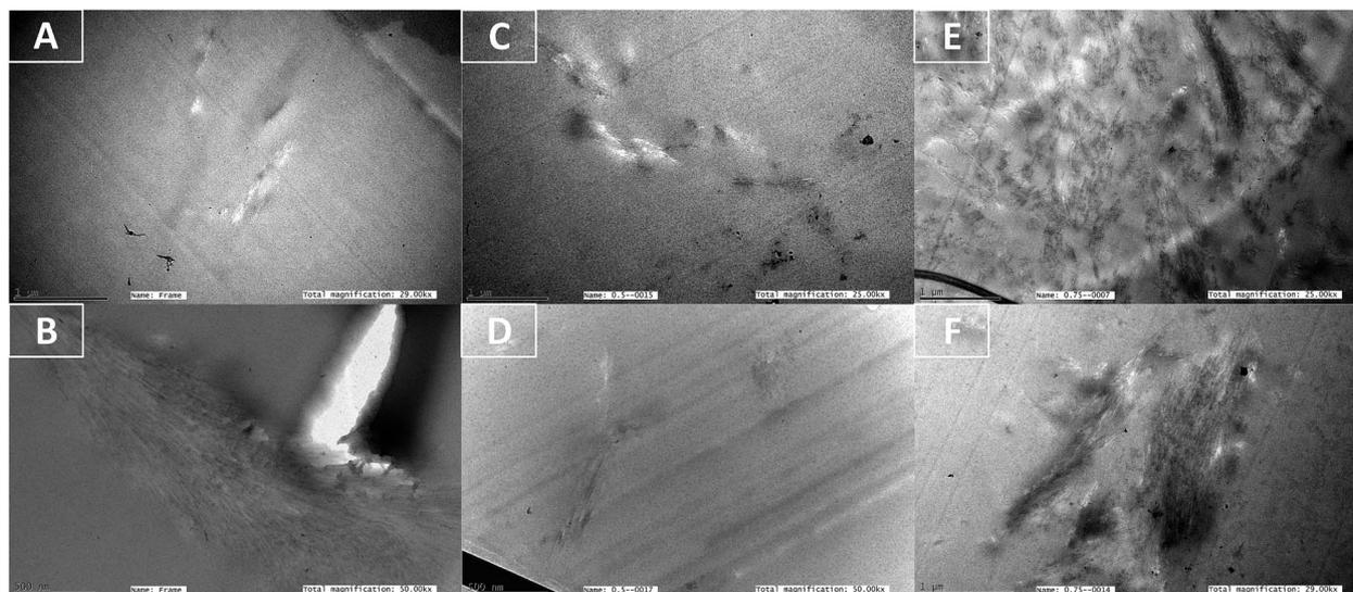
Fig. 5 TEM micrographs of epoxy CNWs nanocomposites: (A & B) 0.25 wt% CNWs, (C & D) 0.5 wt% CNWs, and (E & F) 0.75 wt% CNWs. The sections were negatively stained with uranyl acetate.
