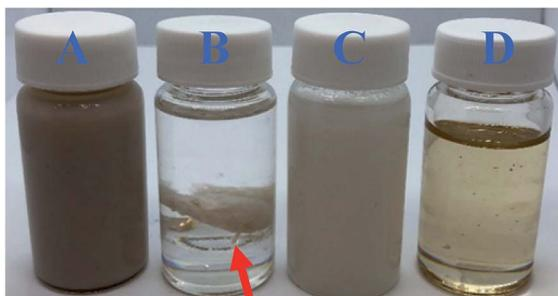
Fig. 2 Epoxy/CNWs solutions through different stages of processing. (A) Opaque CNWs-water suspension, (B) CNWs-water suspension, epoxy (DGEBA) and ethanol mixture at room temperature. The interface due to insolubility of epoxy with the rest of the solution is indicated by the red arrow. (C) The solution in (B) heated above 60 °C and stirred for a brief period. (D) Epoxy-CNWs solution post stirring and after the evaporation of ethanol and water; the high degree of transparency is visible.
