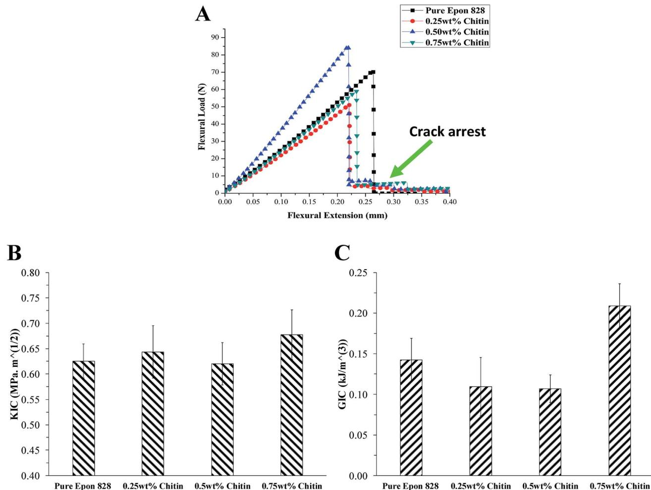
Fig. 7 (A) Flexure load–extension curves from SENB testing. Crack arrest upon initiation of first major fracture is clearly seen in composites of epoxy with CNWs. (B)  $K_{1C}$  and (C)  $G_{1C}$ .
