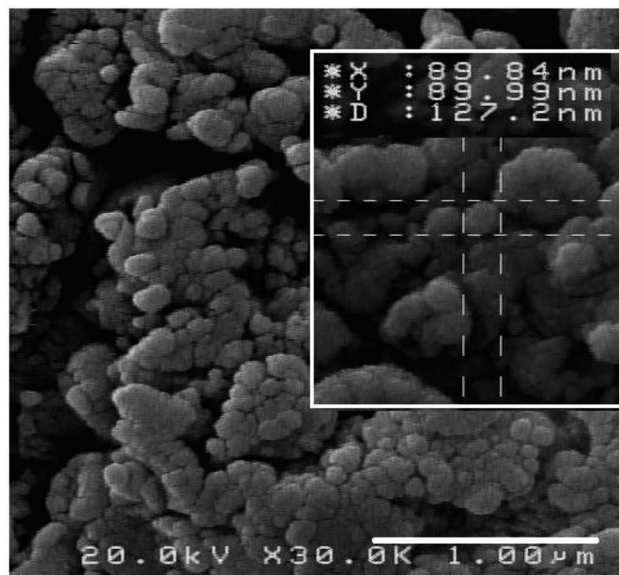
Fig. 1 Scanning electron microscopy image of the synthesized g-C 3 N 4 .
