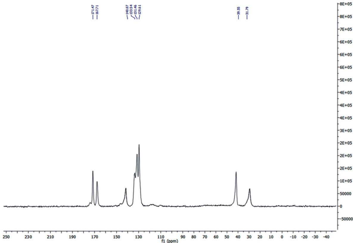
Fig. 3 Solid state <sup>13</sup>C MAS NMR spectrum of S-IRMOF-3.
