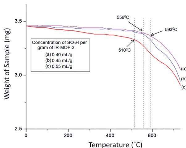
Fig. 8 Effect of SO<sub>3</sub>H content on thermal stability of catalyst.
