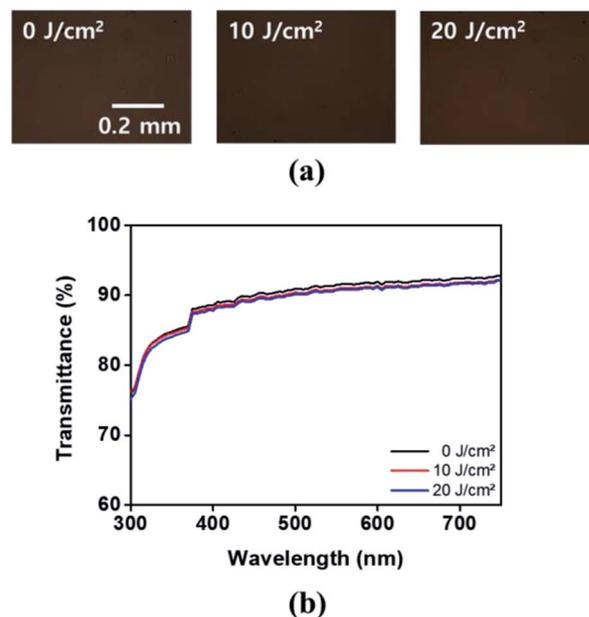
Fig. 10 (a) Orthoscopic POM images of the LC cells made with PPH100 films and (b) UV-Vis transmittance spectra of PPH100 films, before ( $0 \text{ J cm}^{-2}$ ) and after UV treatment at  $10 \text{ J cm}^{-2}$  and  $20 \text{ J cm}^{-2}$ , respectively.
