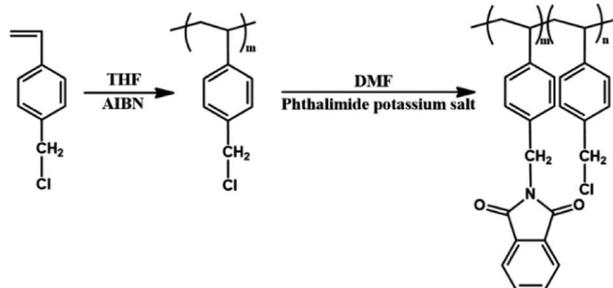
Fig. 1 Synthetic route for phthalimide modified polystyrene (PPH#).
