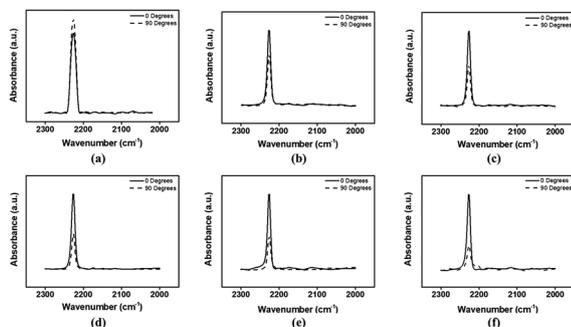
Fig. 7 FT-IR dichroic spectra of LC silicon wafer cells fabricated with rubbed (a) polystyrene, (b) PPH20, (c) PPH40, (d) PPH60, (e) PPH80, and (f) PPH100 films detecting nitrile bond ( $C\equiv N$ ) of 5CB.
