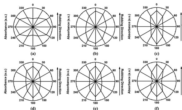
Fig. 8 Polar diagram of specific vibrational IR peaks of nitrile ( $C\equiv N$ ) of 5CB in LC silicon wafer cells fabricated with rubbed (a) polystyrene, (b) PPH20, (c) PPH40, (d) PPH60, (e) PPH80, and (f) PPH100 films measured as a function of rotational angle of polarizer.
