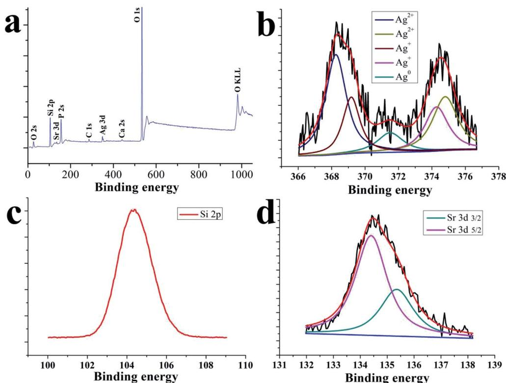
Fig. 4 XPS general spectrum of the surface of the SSAgHA/TNT coating.
