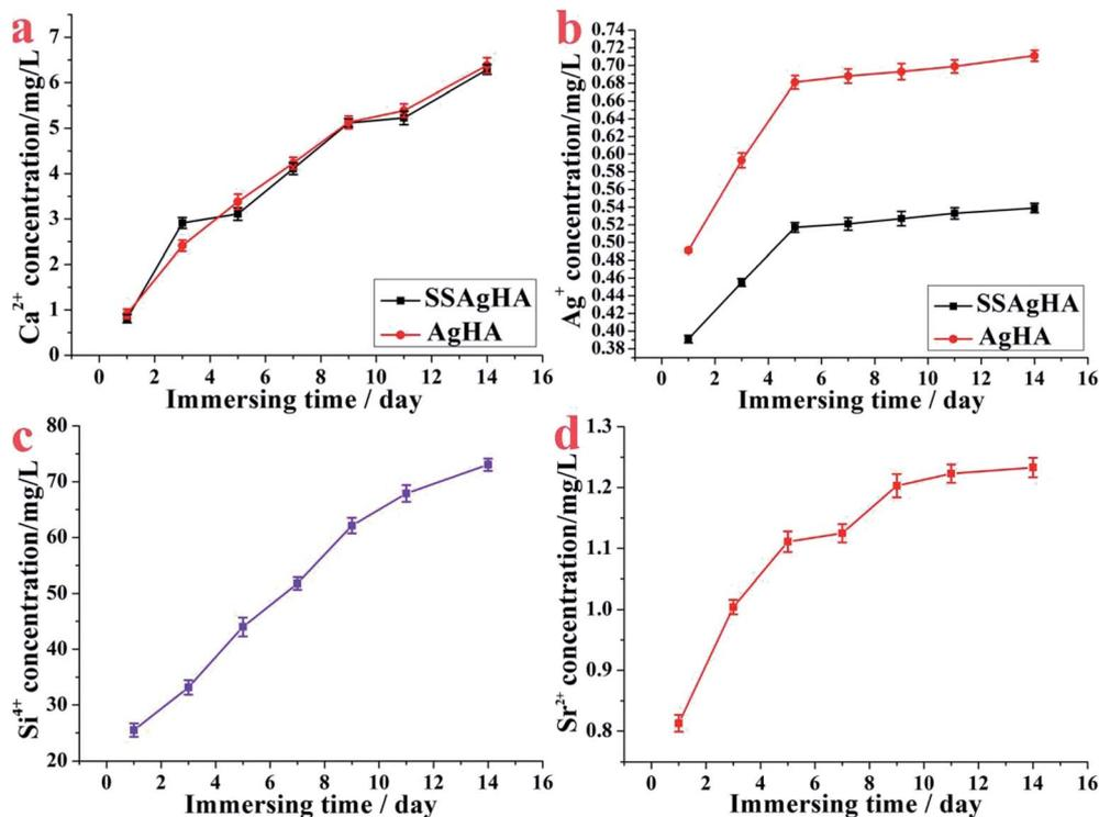
Fig. 8 Amounts of delivered Ca<sup>2+</sup>, Ag<sup>+</sup>, Sr<sup>2+</sup> and Si<sup>4+</sup> species per surface area released from the SSAgHA/TNT coating under static incubation at 37 °C in PBS.
