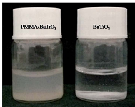
Fig. 9 Suspensions of PMMA/BaTiO 3 and BaTiO 3 particles after sitting for 3 h.
