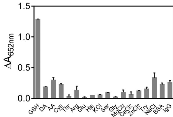
Fig. 7 Selectivity of  $\text{Mn}_3\text{O}_4$ -TMB system for GSH over other potential interferences. Reaction conditions:  $0.416 \text{ mM}$  TMB,  $10 \mu\text{g mL}^{-1}$   $\text{Mn}_3\text{O}_4$  microspheres,  $\text{pH} 4.5$  and room temperature. Concentrations of the tested substances:  $600 \mu\text{M}$ , except for  $60 \mu\text{M}$  GSH,  $6 \mu\text{M}$  DA,  $6 \mu\text{M}$  Cys,  $20 \mu\text{M}$  AA,  $1 \text{ mg mL}^{-1}$  of BSA, and  $1 \text{ mg mL}^{-1}$  IgG.
