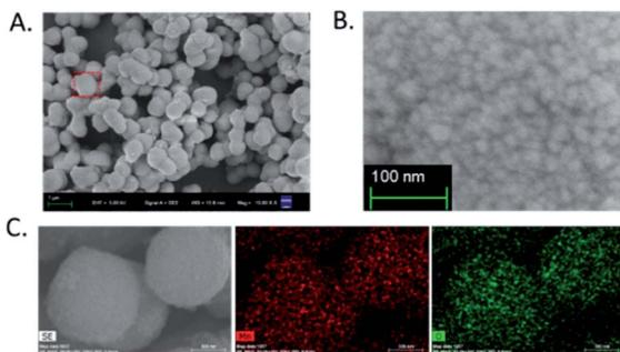
Fig. 1 (A) SEM image of  $\text{Mn}_3\text{O}_4$  microspheres. (B) High-magnification SEM image of an individual  $\text{Mn}_3\text{O}_4$  microsphere. (C) Elemental mapping images of Mn and O in  $\text{Mn}_3\text{O}_4$  microspheres.
