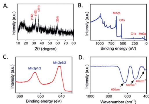
Fig. 2 (A) XRD patterns of  $\text{Mn}_3\text{O}_4$  microspheres. (B) XPS spectrum of  $\text{Mn}_3\text{O}_4$  microspheres. (C) Mn 2p peak of  $\text{Mn}_3\text{O}_4$  microspheres. (D) FT-IR spectrum of  $\text{Mn}_3\text{O}_4$  microspheres.
