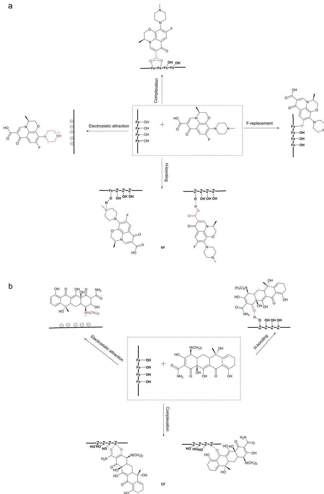
Fig. 7 Possible adsorption mechanisms for LEV (a) and TC (b).
