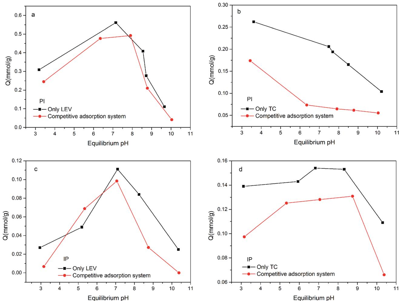
Fig. 6 The adsorption amount in the single and competitive systems: (a) LEV adsorption amount by PI; (b) TC adsorption amount by PI; (c) LEV adsorption amount by IP; (d) TC adsorption amount by IP.
