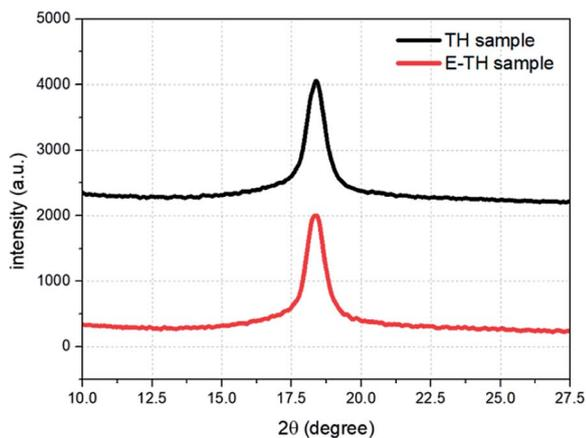
Fig. 5 X-ray spectra for two annealed samples.
