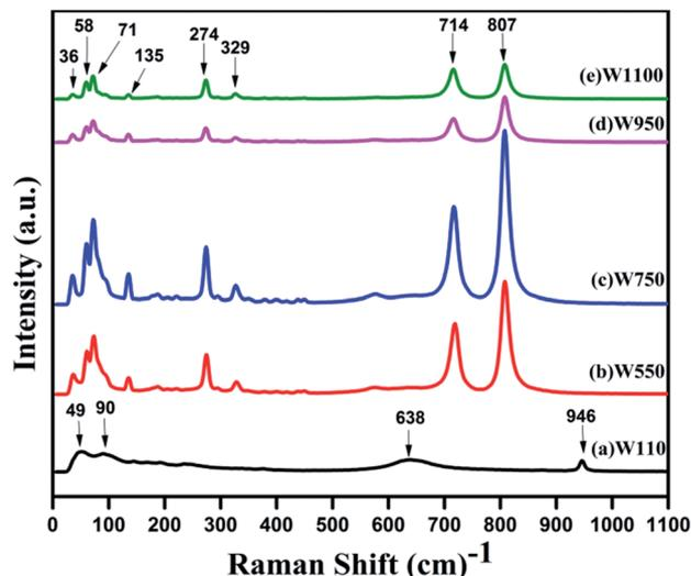
Fig. 7 Raman spectra for different annealed samples (a) W110, (b) W550, (c) W750, (d) W950, and (e) W1100. The characteristic Raman modes of  $\text{WO}_3$  are indicated in each case. The peak positions marked with arrows in (a) show orthorhombic phase of  $\text{WO}_3 \cdot \text{H}_2\text{O}$ .
