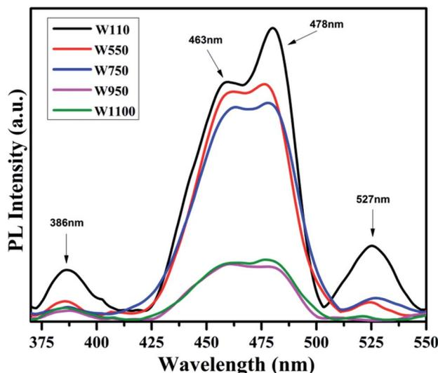
Fig. 9 PL spectra of the annealed samples recorded at  $\lambda_{\text{exc}} = 320$  nm giving emission at 386 nm due to resonant states in the CB; emission at 463 nm due to band–band transition and emission peaks at 478 nm and 527 nm due to donor like states present within band gap.
