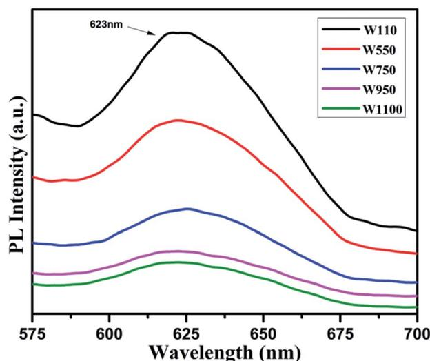
Fig. 10 PL spectra of the annealed samples recorded at  $\lambda_{\text{exc}} = 450$  nm. The emission is due to optical transition from different oxygen vacancy states ( $\text{V}_\text{O}^{2+}/\text{V}_\text{O}^{1+}$ ).
