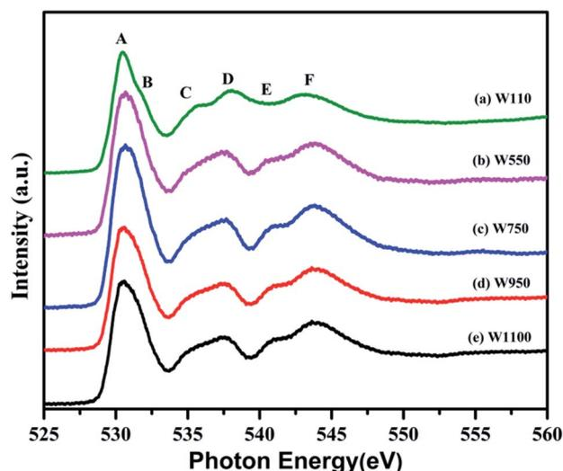
Fig. 16 O-K edge fine structure of prepared samples (a) W110, (b) W550, (c) W750, (d) W950 and (e) W1100. Disappearance of peaks B and C in spectra (b)–(e) reflects the change in hybridization between O 2p and W 5d orbitals with structural phase transformation.
