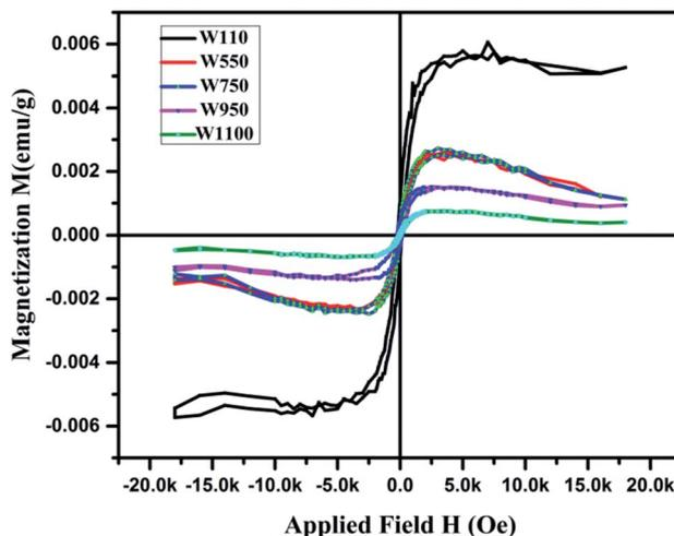
Fig. 13 Typical hysteresis loops of the annealed samples at 300 K.
