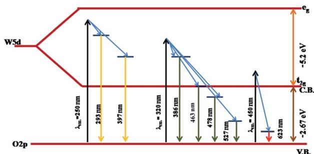
Fig. 11 Band diagram of  $WO_3$  showing NUV emissions (293 nm, 397 nm, and 386 nm) due to resonant states of oxygen vacancies, band to band transition (463 nm), emission due to midgap defect states along (+2/0) transition along crystallographic axes  $b$  and  $c$  (478 nm), along (+2/+1) transition along crystallographic axes  $b, c$  (527 nm) and axes  $a$  (623 nm).
