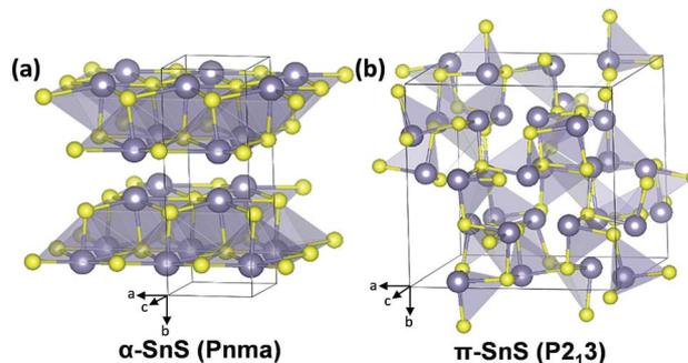
Fig. 1 Tilted views of the assigned crystal structures and space groups for (a) the  $\alpha$ -orthorhombic-SnS and (b) the  $\pi$ -cubic-SnS polymorph (Sn, grey; S, yellow).<sup>32</sup>
