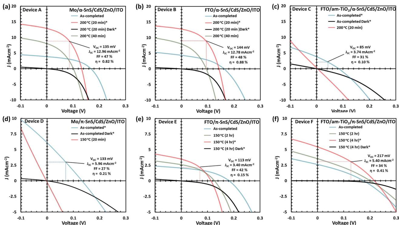
Fig. 7  $J$ - $V$  characteristics in the dark and under simulated AM 1.5 G illumination for the as-completed and after subsequent hot plate treatment of the solar cells A-F (a-f). Only the PV device parameters, for the highest pixel efficiencies and optimized conditions, are presented.
