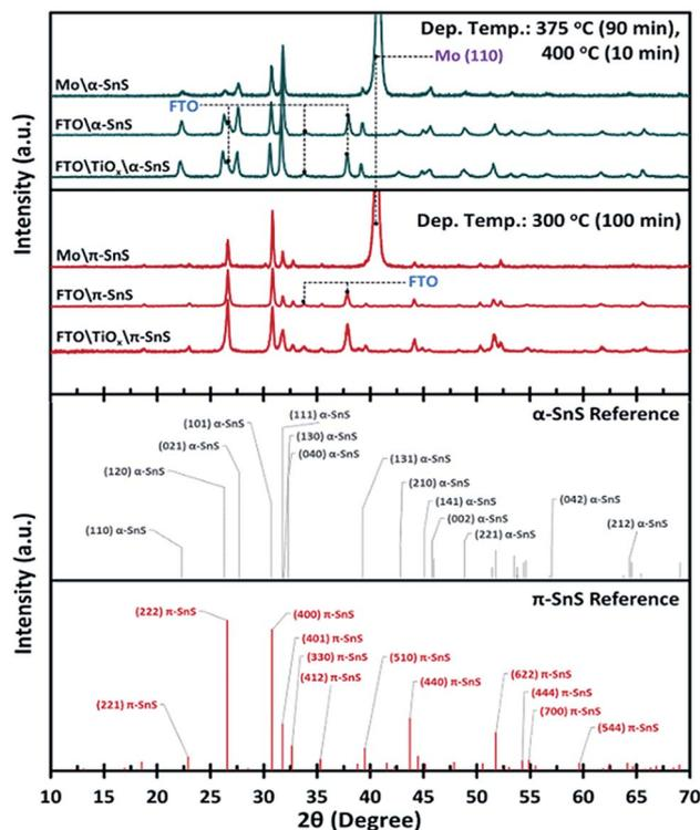
Fig. 2 Comparison of XRD patterns, with assigned reference peaks, for selectively deposited  $\alpha$ - and  $\pi$ -SnS thin films deposited onto Mo, FTO or am-TiO<sub>x</sub>/FTO substrates by AA-CVD using the Sn(II) thio-ureide complex as a single source precursor.
