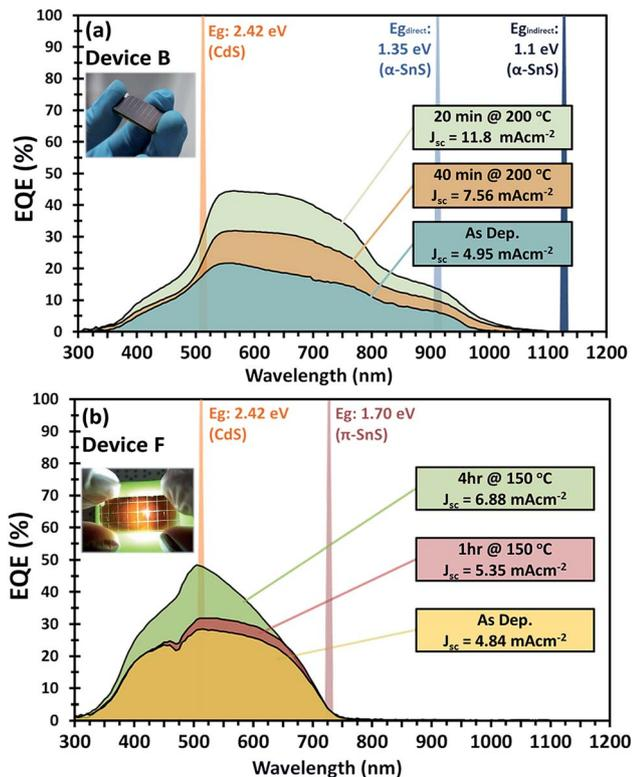
Fig. 8 External quantum efficiency (EQE) vs. photon wavelength for (a) device B consisting of FTO/ $\alpha$ -SnS/CdS/ZnO/ITO and (b) device F consisting of FTO/am-TiO<sub>x</sub>/ $\pi$ -SnS/CdS/ZnO/ITO. The EQE measurements after consecutive hot plate annealing treatments are presented. Inset are photographic images of each device respectively.
