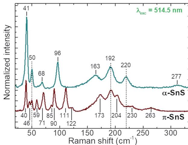
Fig. 3 Comparison of Raman spectra for  $\alpha$ -SnS and  $\pi$ -SnS samples deposited onto FTO substrates, using a 514.5 nm laser wavelength. For convenience, the spectra were normalized to the peak at  $192 \text{ cm}^{-1}$  and shifted along the Y axis.
