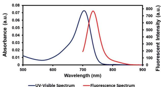
Fig. 1 UV-vis-NIR absorption and fluorescent spectra of AZB-IMC<sub>2</sub> (2.9 μM) excited at 670 nm in DMSO.Table 1 Photophysical properties of AZB-IMC<sub>2</sub>
