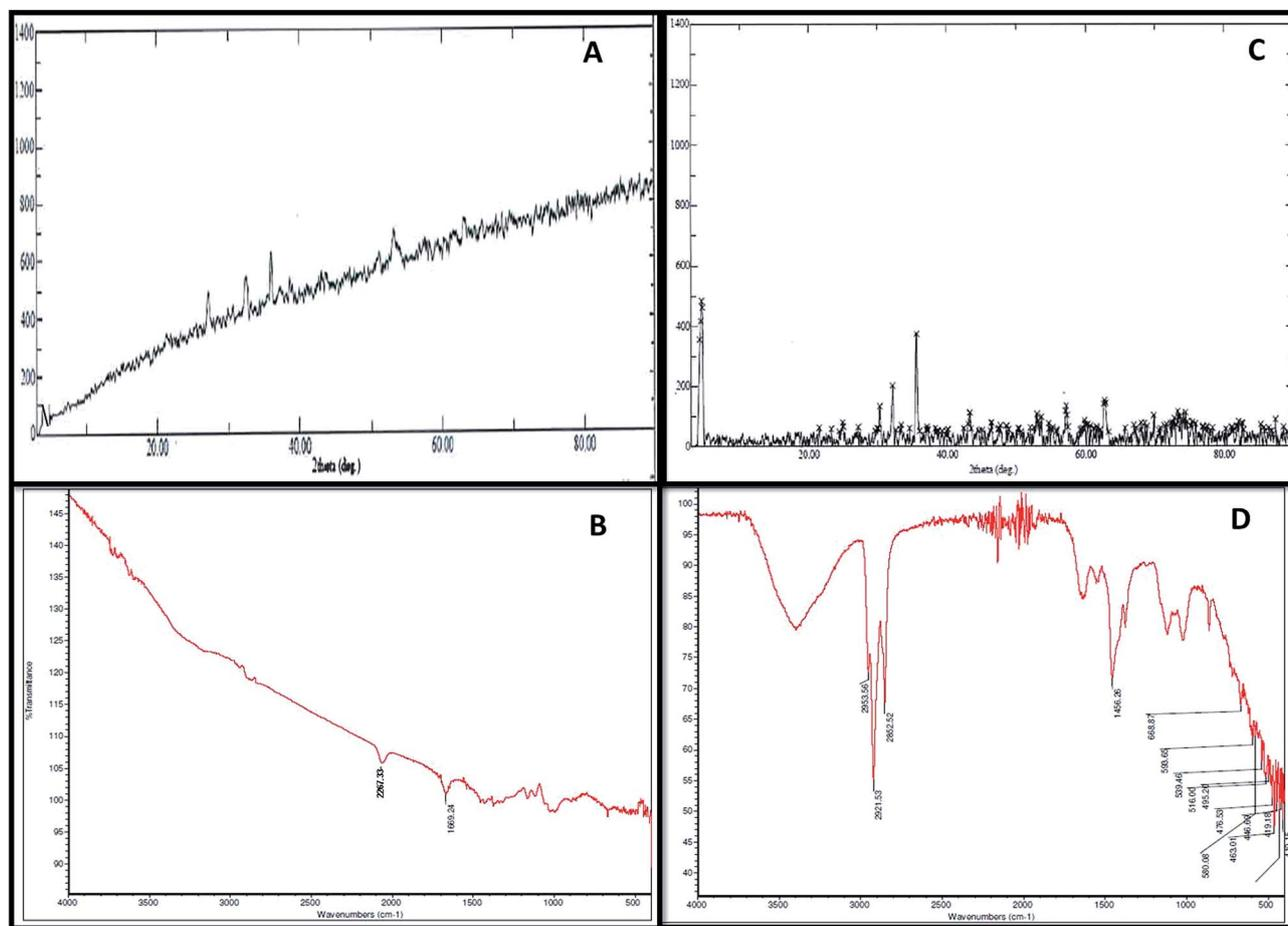
Fig. 3 The corrosive chemical composition produced in the abiotic and biotic systems illustrated by FT-IR and XRD spectra. (A and B) Represent the FT-IR and XRD results for the abiotic system, respectively. (C and D) Show the FT-IR and XRD results for the biotic system, respectively.
