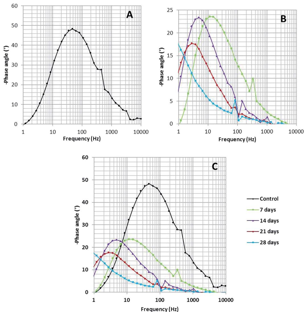
Fig. 6 The Bode phase spectra of (A) the abiotic system and (B) the biotic system on 7<sup>th</sup>, 14<sup>th</sup>, 21<sup>st</sup> and 28<sup>th</sup> days; (C) depicts the comparison of the abiotic and biotic systems.
