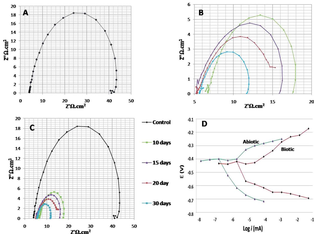
Fig. 4 The Nyquist and Tafel spectra. (A) Illustrates the spectra of the abiotic system, (B) illustrates the spectra of the biotic system for 7<sup>th</sup>, 14<sup>th</sup>, 21<sup>st</sup> and 28<sup>th</sup> days, (C) shows the combined spectra for both abiotic and biotic systems, and (D) elucidates the Tafel plots of the abiotic and biotic systems (on the 28<sup>th</sup> day).
