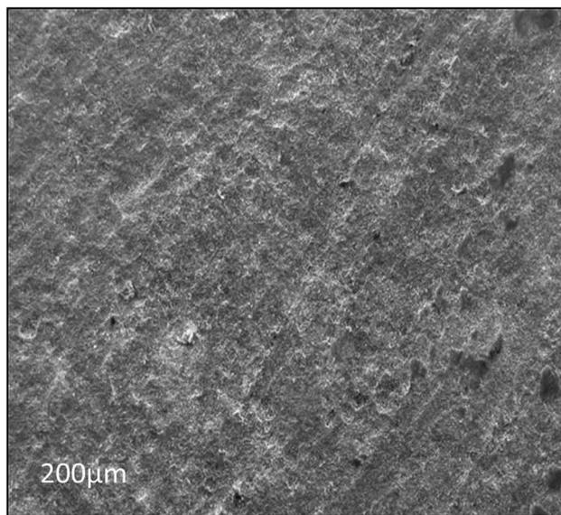
Fig. 11 The SEM image of the abiotic system, showing that the metal coupon surface is cleaned after the 28<sup>th</sup> day of incubation.
