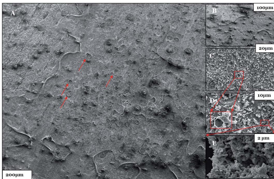
Fig. 12 (A–E) The SEM micrographs of the biotic system after the 28<sup>th</sup> day of incubation. Pit holes are shown by the red arrows and boxes.
