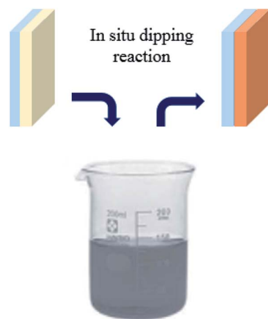
Scheme 1 Sequential deposition method; dipping the PbBr 2 film into MABr solution.
