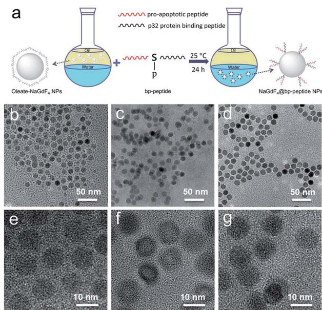
Fig. 1 The schematic representation of transfer and functionalization of OA-coated NaGdF<sub>4</sub> nanoparticles by bp-peptide (a), and TEM and HRTEM of NaGdF<sub>4</sub> nanoparticles (b and e), NaGdF<sub>4</sub>@bp-peptide NPs (c and f) and NaGdF<sub>4</sub>@CPP NPs (d and g), respectively.
