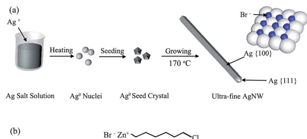
Fig. 9 (a) Schematic representation of the proposed growth mechanism of AgNWs, (b) molecular structure of the 6CHZB.
