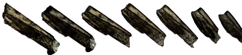
Fig. 2 An image depicting successive partial dissolutions of one crystal of compound 1 from the series containing 4.0 mol% of compound 2. From left to right, the first crystal is the initial crystal before any dissolution media was applied, continuing progressively to the final crystal, at which point no more dissolution media was applied.
